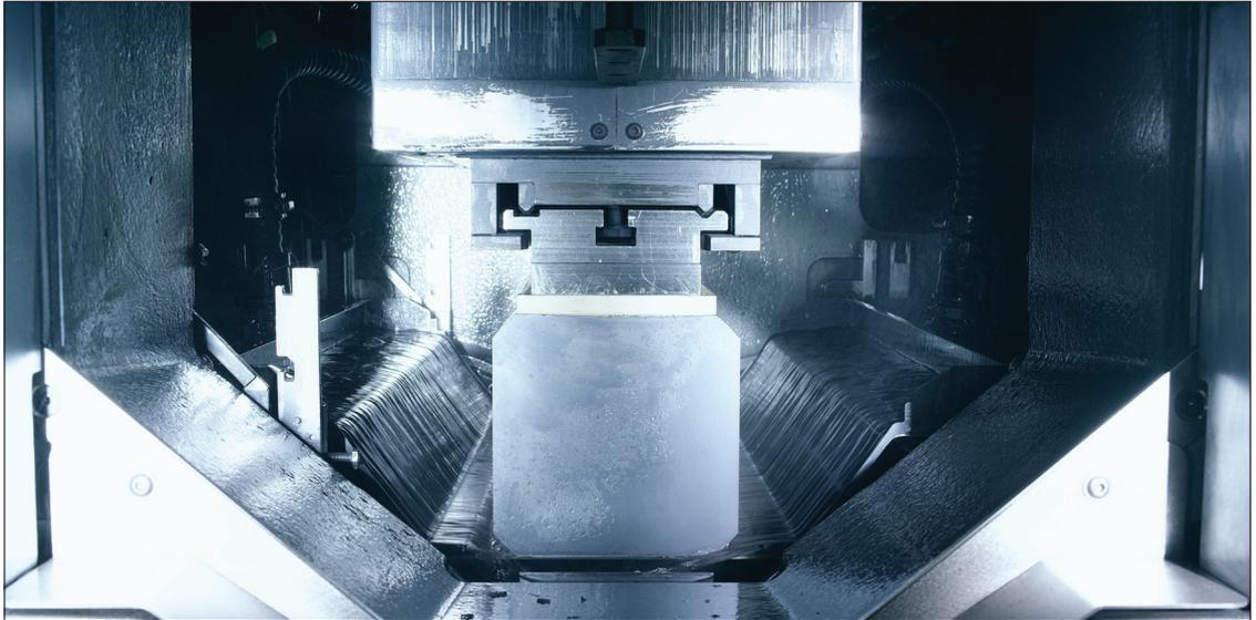
factor is that, even with the thinnest wires, the sensitive control reliably maintains the extremely fine line between optimum yield and the risk of a wire break: the wire tension remains constant up to 0.5 N. Without exerting any additional stress on the wire, the cyclic acceleration and braking processes can be configured more dynamically and in addition, a higher cutting speed can be maintained – up to 30 m/s.
