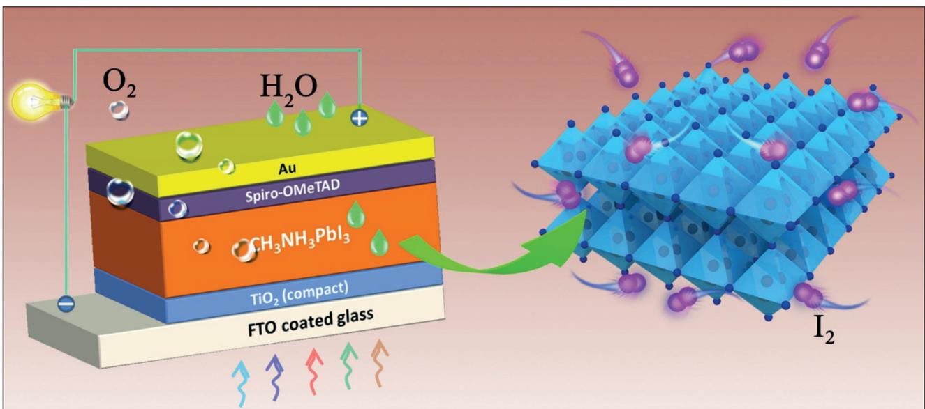
The schematic drawing showing that various factors (e.g., moisture, oxygen, light illumination, applied electric field, etc.) during the operation of MAPbI<sub>3</sub> perovskite solar cells can generate iodine, which leads to degradation of solar cells.
