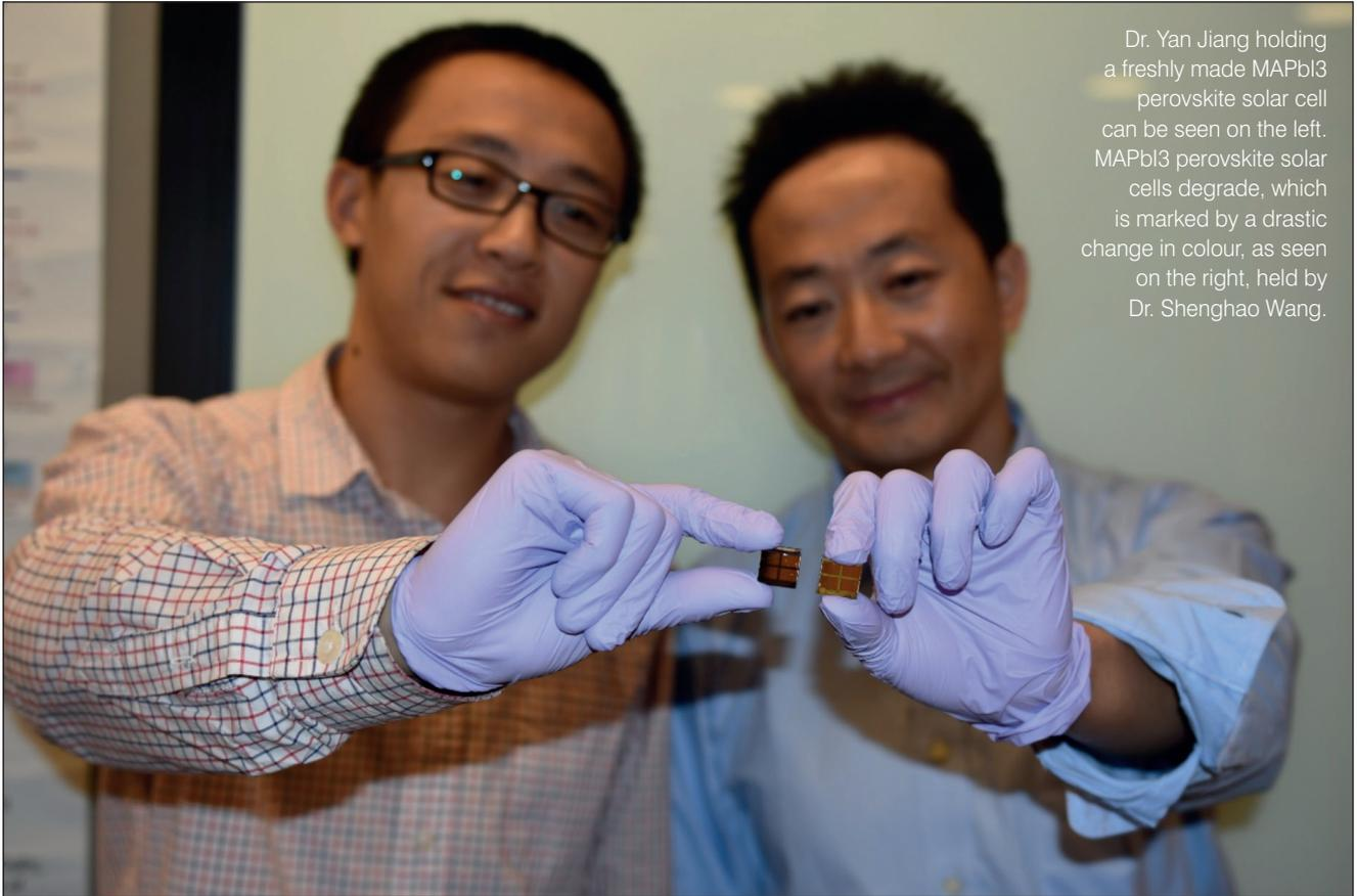
Dr. Yan Jiang holding a freshly made MAPbI<sub>3</sub> perovskite solar cell can be seen on the left. MAPbI<sub>3</sub> perovskite solar cells degrade, which is marked by a drastic change in colour, as seen on the right, held by Dr. Shenghao Wang.
