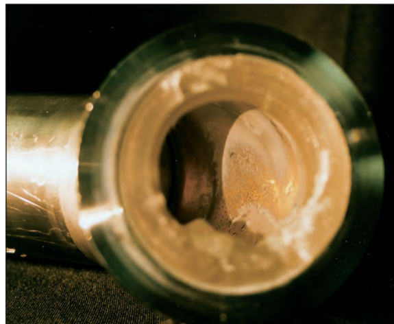
Left: Fig. 1: Illustrates the reduction in tube cross section due to aluminum chloride build up in an insufficiently heated tube
