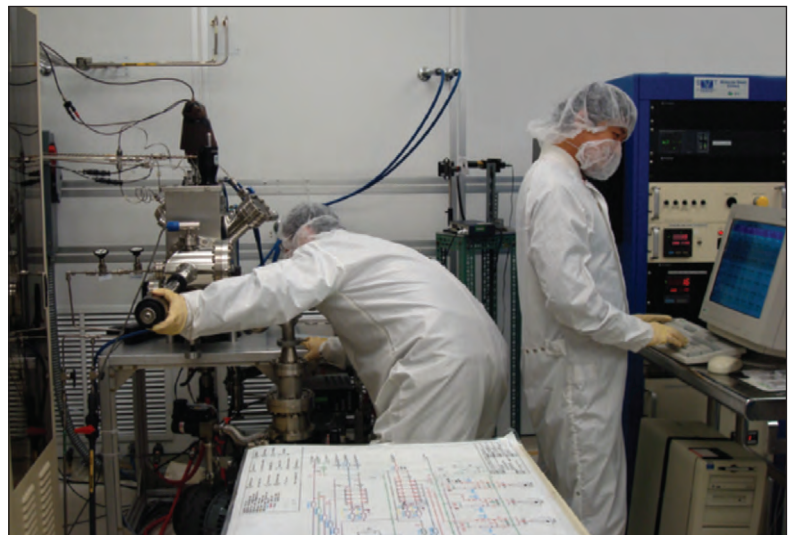
The MOCVD reactor at Virginia Commonwealth University has been used for the InGaN-based LED study. This custom-designed system utilizes a gas delivery system manufactured by Emcore Corporation and a vertical deposition chamber, equipped with an in-situ reflectance monitor that enables the measurement and control of film thickness during epitaxy
