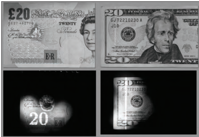
Figure 3: Currency anti-counterfeiting measures incorporate UV threads imbedded into a currency in order to validate the authenticity and quickly detect forgeries. The currency is illuminated with a 365nm UV LED.
