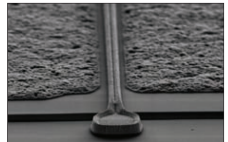
The AlInN/GaN HEMT fabricated by ETH Zürich and EPFL features Ni/Au T-shaped 100 nm gates. Credit: ETH Zurich
