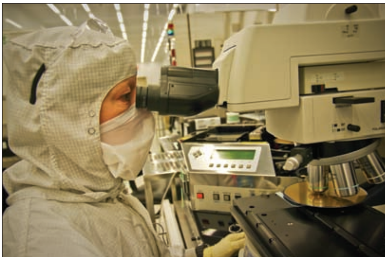
Quality check on a wafer being fabricated at TriQuint's Hillsboro, Oregon facility
