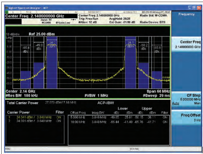
Figure 2. The AWB7227 amplifier is capable of supporting multiple carriers, a feature that can be useful in certain deployment scenarios. Each carrier represents a group of users operating at a particular frequency. Here, the device has been subjected to 2 WCDMA Test Mode 1, 64 DPCH carriers at maximum separation
