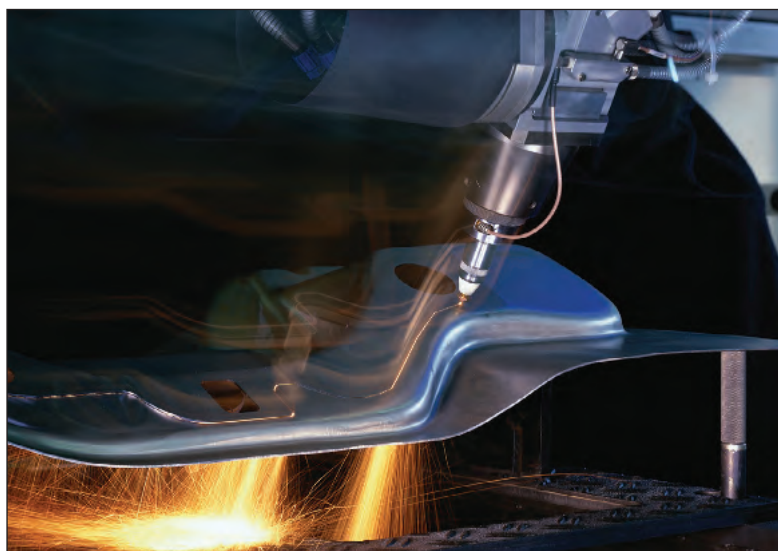
Fig 1: Fiber coupled diode lasers (left) are the enabling technology for many of today's state of the art, high-efficiency industrial laser systems (right). High-efficiency diode lasers with narrow, stable spectral lines are needed for further improvements in the brightness of such systems. Credit: FBH/Immerz, TRUMPF
