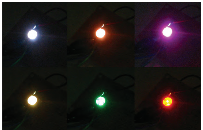
Figure 4. Wide range of colors emitted by a stacked LED
