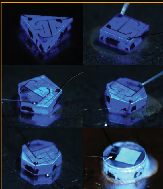
Figure 1. Laser-micro- machined LED chips
