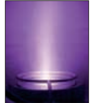
Plasma sources enable enhanced evaporation at lower process temperatures
