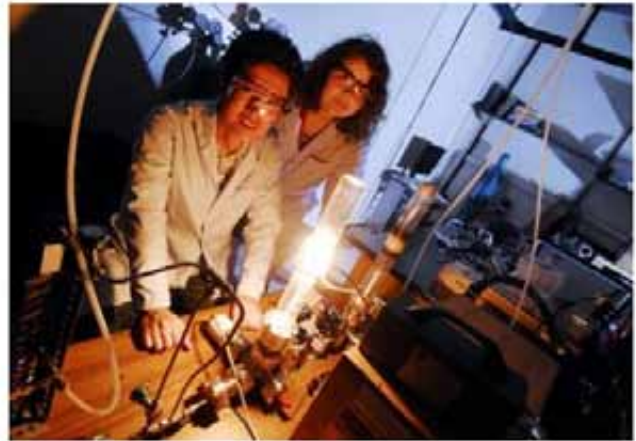
Georgia Tech graduate student Baiqian Zhang and undergraduate student Holly Tinkey observe a high-temperature furnace used to produce epitaxial graphene on a SiC wafer
