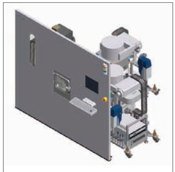
Simple cluster configuration with load lock, central handler and single process modules for sputter, etch
