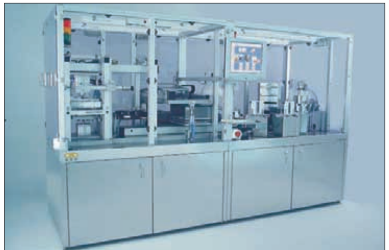
Figure 2: The fully automated EVG850 Temporary Bonder with dry-film Lamination
