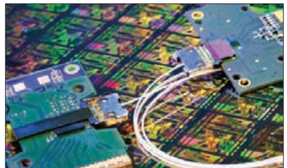
Klaus Ploog pointed out that optical approaches could help to improve data communication within computer hardware. Intel has been at the forefront of efforts to do this, developing InP-on-silicon hybrid lasers. In this image of a 50 Gbit/s silicon photonics link, the transmit module (left) sends laser light from the silicon chip at the center of the green board, which then travels through optical fiber to the receiver module (right), where a second silicon chip detects the data on the laser and converts it back into an electrical signal. Credit: Intel
