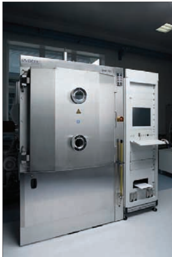
Typical box coater batch system – available in chamber sizes from 0.5 to 2 m
