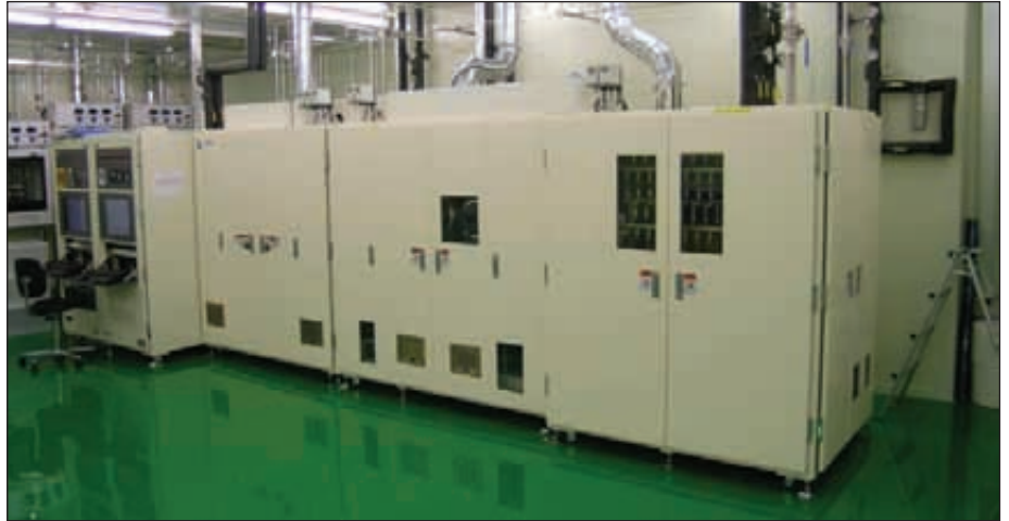
LED structures were produced on a Taiyo Nippon Sanso SR-4000 tool that has a capacity of three 2-inch wafers
