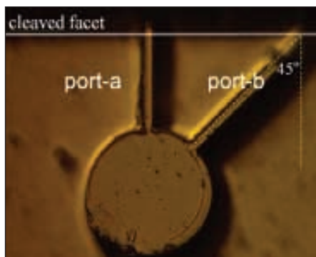
Figure 1. Microscope image of a cylinder microlaser with two output waveguides cleaved for testing
