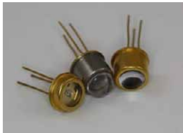
Figure: SETi's UVTOP LEDs
