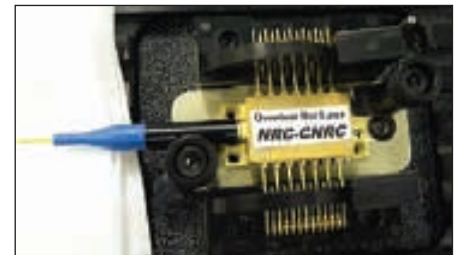
Fiber-pigtailed packaged, quantum-dot, distributed feedback laser
