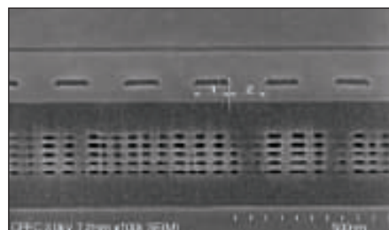
A cross-sectional scanning electron microscope image of the quantum-dot, distributed feedback laser structure showing the five-layer quantum-dot core and the floating grating. Distances (1) and (2) are 117 nm and 119 nm, respectively
