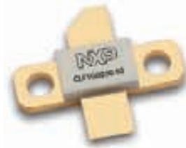
The first product in NXP's GaN power product portfolio is the CLF1G0530-50, a broadband amplifier spanning the 500-3000 MHz range that has a nominal P1dB of 50W
