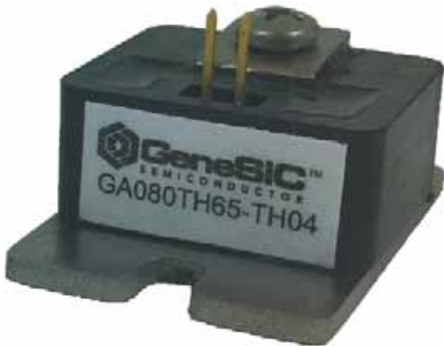
Figure. GeneSiC silicon carbide thyristor
