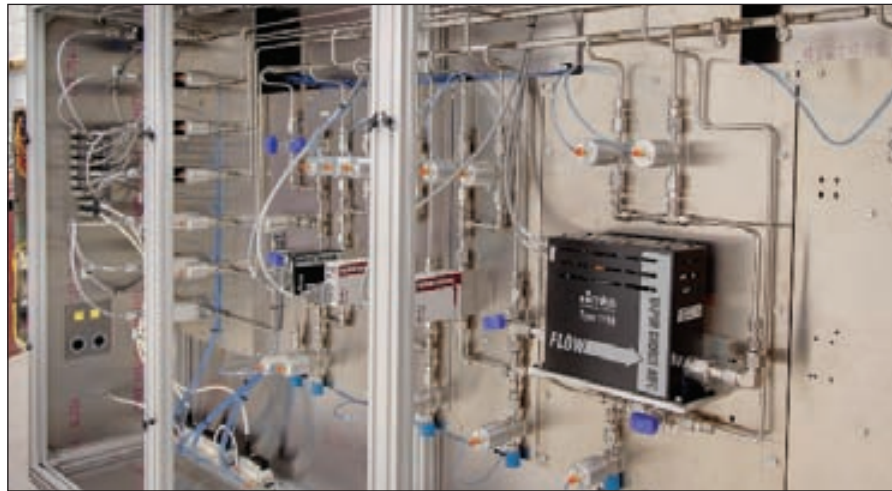
Metalorganic vapour delivery system used for the Meaglow reactor. Operating at close to 1 Torr carrier gases are not required for most metalorganics - greatly simplifying the vapour delivery system compared to MOCVD
