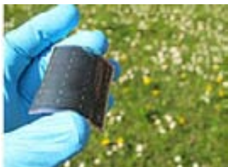
Caption: Flexible thin film CIGS solar cell on polymer substrate developed at Empa (Copyright: Empa)
