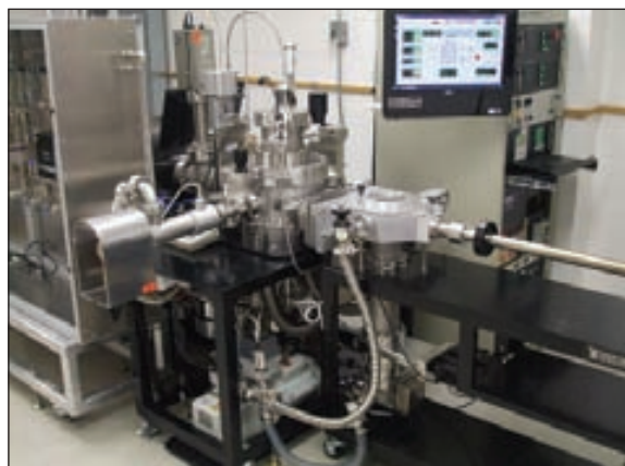
A wide view of the prototype Meaglow reactor, showing the UHV central growth chamber with load lock, RGA and RHEED analysis chamber, MO delivery system (on left), control electronics (on right)
