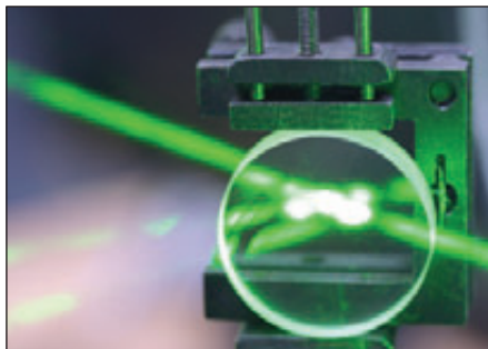
Corning's semi-polar lasers deliver a 60 mW continuous-wave output at 519 nm
