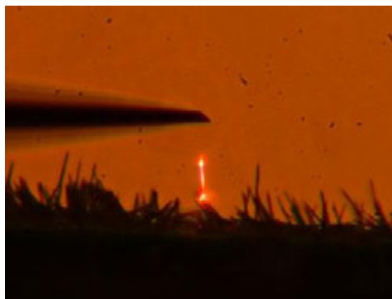
Optically pumped GaN nanowire laser shown
