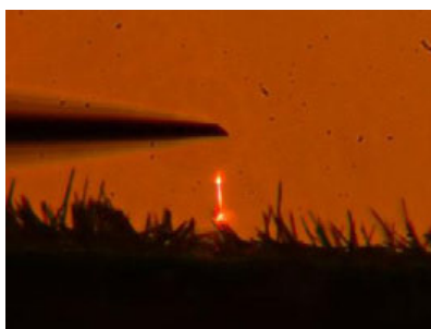
Optically pumped GaN nanowire laser shown glowing orange. The actual laser output is UV
