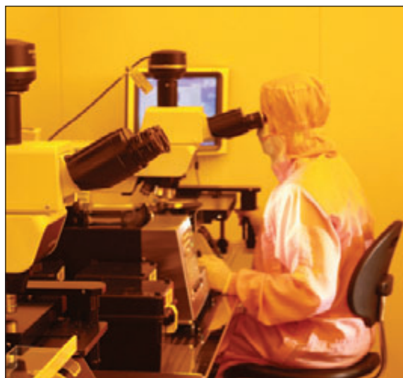
Optical inspection of 6-inch GaAs wafers in fab B
