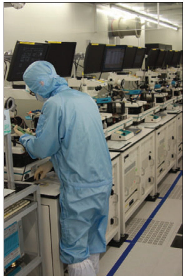
Right: A vast army of tools test production die. For a premium, customers can have every single die of theirs tested - the other option is to have a carefully selected proportion of these chips examined prior to shipment
