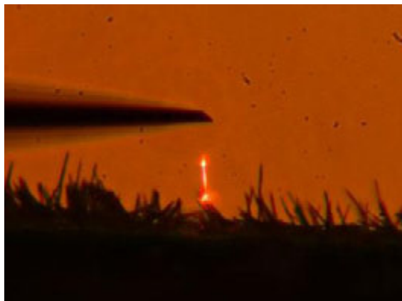
Optically pumped GaN nanowire laser shown glowing orange. The actual laser output is UV ( \approx 370 nm) and invisible to the unaided eye. The length of the lasing nanowire is roughly 10
