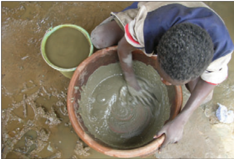
Figure 4. Artisan miner in Tanzania mixing mercury by hand with crushed ore to extract gold. (Photo credit: Antony Benham, NERC)
