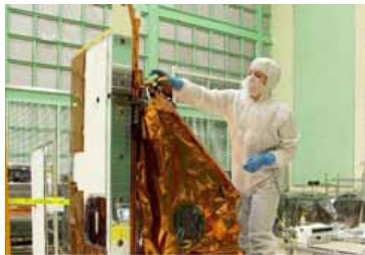
Aleksandra Bogunovic reaches across the instrument to affix the corners of a Multi-Layer Insulation blanket to the TIRS instrument (Credit: NASA Goddard/Rebecca Roth)
