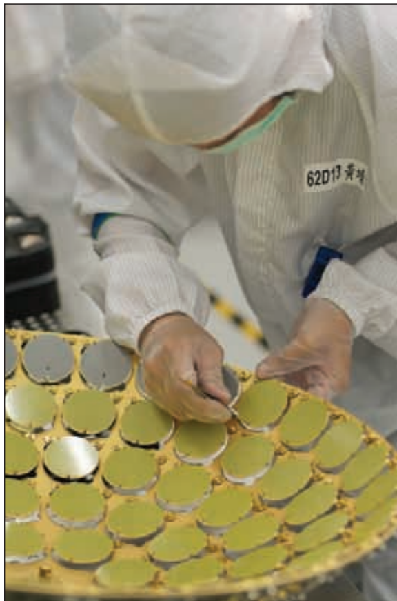
An Epistar technician loading and unloading the LED wafers in a tool for the metallization process
