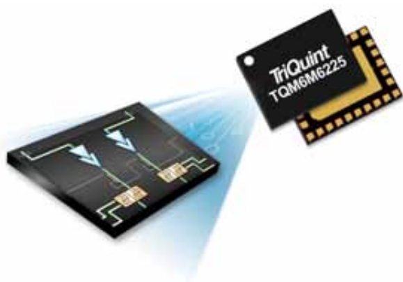
TriQuint's TRITIUM Duo™: Industry's First Dual-Band Power Amplifier Module
