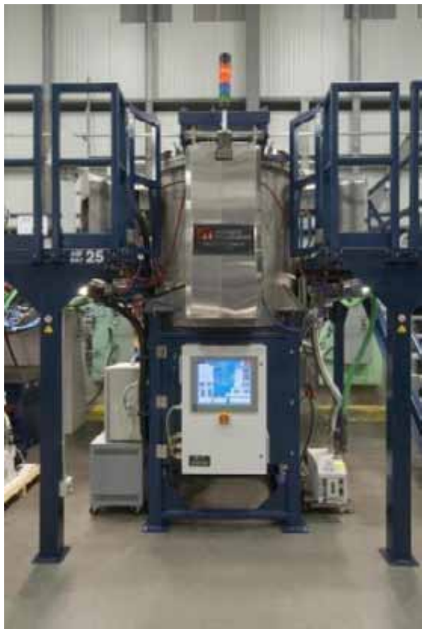
GT's ASF sapphire growth furnace which utilises HEM for producing high quality boules and cores suitable for the LED industry and other industries requiring high quality material
