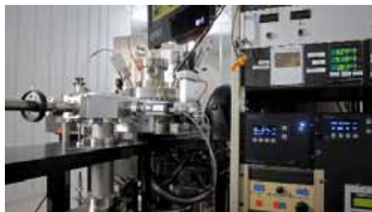
Patented Migration Enhanced Afterglow (MEAglow) Reactor that grows the InN wafer
