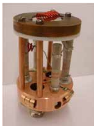
The probe head used to send radio-frequency pulses onto the coil used for pulsed spin manipulation of a GaAs sample. (Credit: Yunpu Li)
