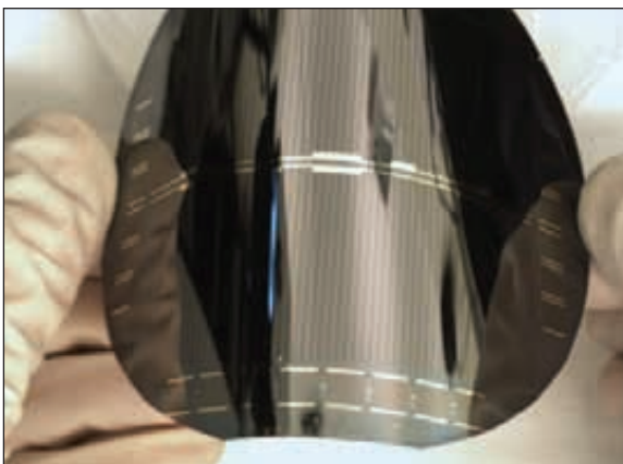
A 4-inch film produced by MicroLink's epitaxial lift-off process features two, 20 cm 2 solar cells on a thin, flexible metal backing
