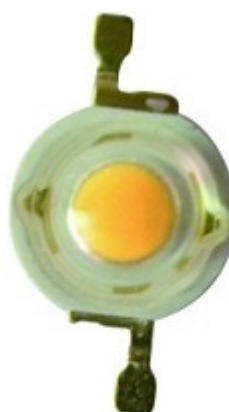
TK-AC01 Produce size: 8mm Color temp.: 2700-6500K Lum: 100-120LM Wattage: 1W Voltage: AC230V/120V
