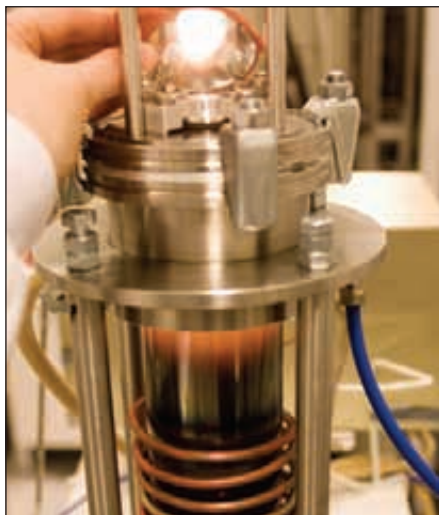
Figure 2. Sublimation growth at 1800 °C is comparable to 2200-2300 °C used in conventional PVT
