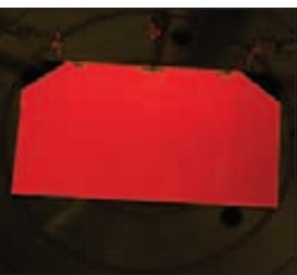
Figure 3. Biasing the top junction so that it produces electroluminescence enables assessments of the uniformity and material quality of this junction
