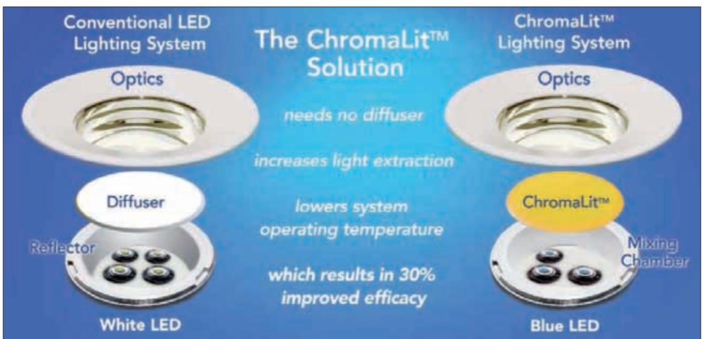
Figure 2. Intematix ChromaLit lighting systems use blue LEDs in a mixing chamber to provide higher system performance and simplification of the optical interface
