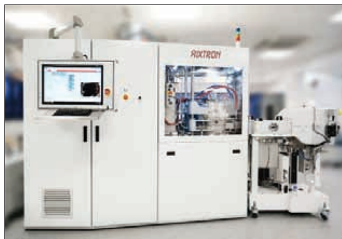
Robot loading is one of the features of Aixtron's BM 300T, which is in the process of internal qualification
