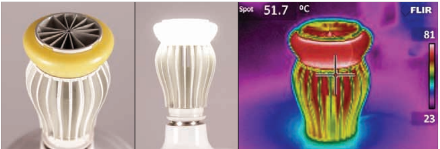
Figure 4. A 75 W equivalent lamp operating in power-off condition (a) and power-on condition (b). The thermal profile of the lamp (c) shows that the remote phosphor is just 82°C
