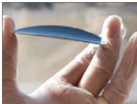
Figure 1: Cubic SiC grown on silicon shows severe bending
