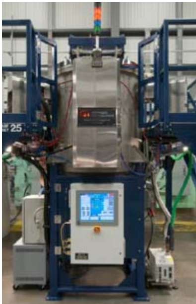
GTAT ASF furnace
