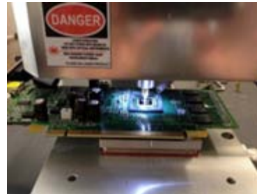
An integrated circuit on a graphics board being prepared on the ASAP-1 IPS in End-point Detection Mode
