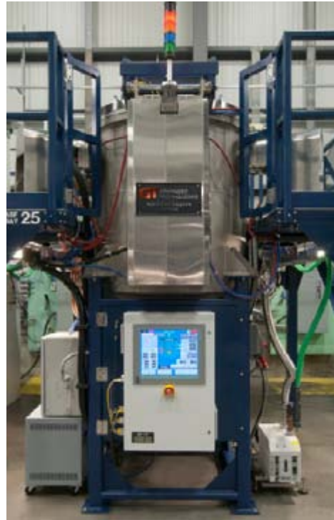
GTAT ASF furnace
