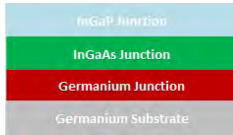
ZTJ solar cell structure
