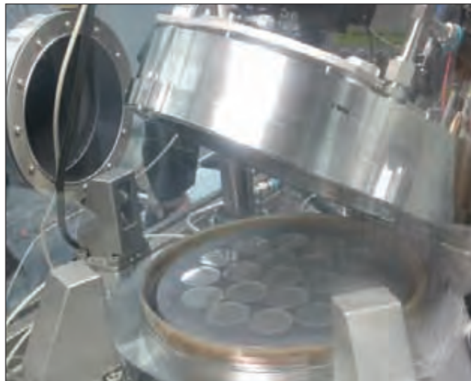
Engineers at IMRE have carried out the development of GaN-on-silicon epitaxial wafers using a modified CCS reactor. (Top left) The Aixtron MOCVD tool being used for the development of GaN-on-silicon product at IMRE-Singapore. (Top right) The usage of the reactor for conventional GaN-on-sapphire 19 x 2-inch mode epitaxy. (Bottom left) The same chamber with a 200 mm, deep-pocket susceptor for GaN-on-silicon epitaxy. (Bottom right) A 150 mm diameter GaN-on-silicon epiwafers, which is also developed at IMRE using the same reactor
