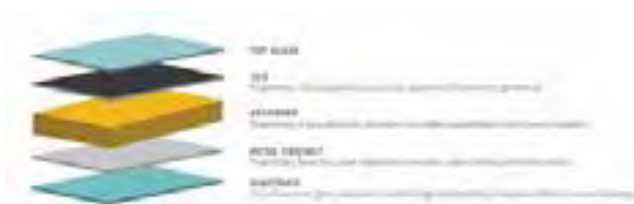
Stion CIGS solar cell structure
