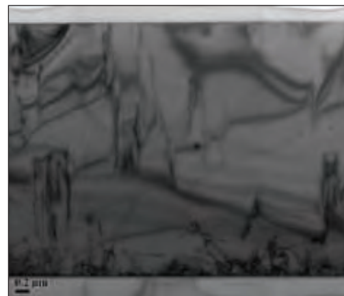
The TEM images shows low temperature RPCVD GaN layers on MOCVD GaN layers; each has a low defect density and good crystalline quality. (The lower image is at a lower magnification)
