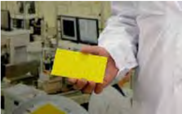
Optogan X10 LED module consisting of 72 items
