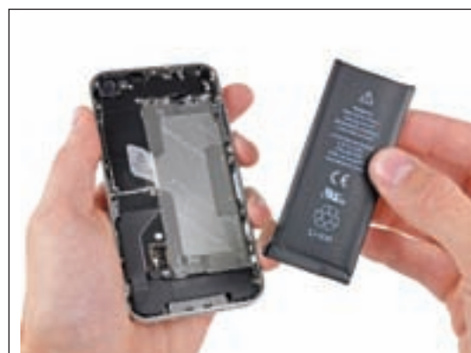
Figure 2: The amount of space available for the RF section in RFFE designs is greatly diminishing, as the battery continues to consume the majority of real estate within a handset
