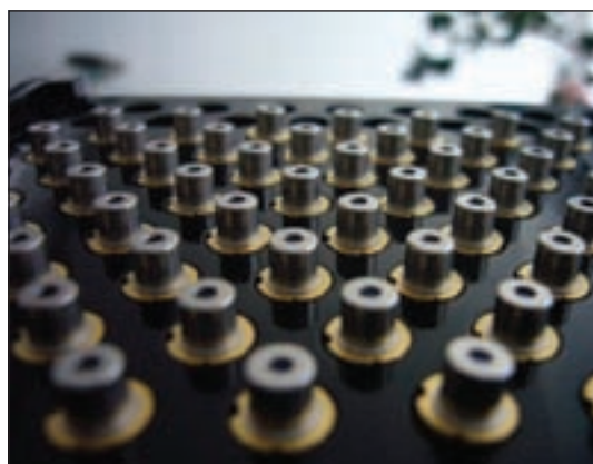
300 mW CW single mode laser diode for use in structured light applications
