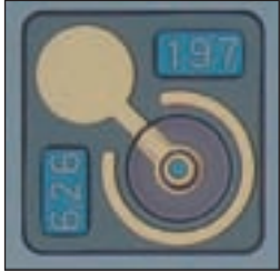
Oclaro has produced a 10 Gbit/s VCSEL chip for use in non-hermetic, high-speed optical interconnects
