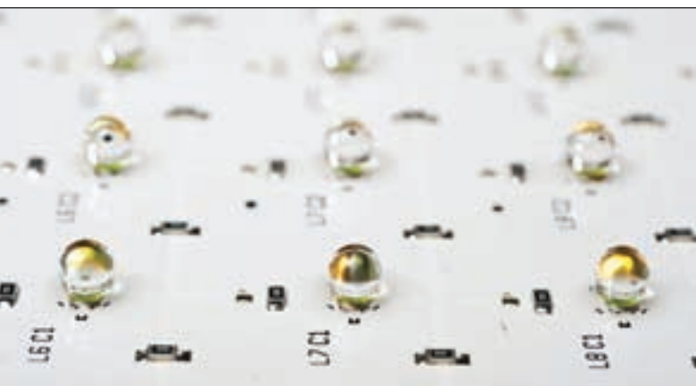
Semprius modules use hundreds of GaAs solar cells with lenses to concentrate light, boosting the efficiency and making the exotic photovoltaic affordable
