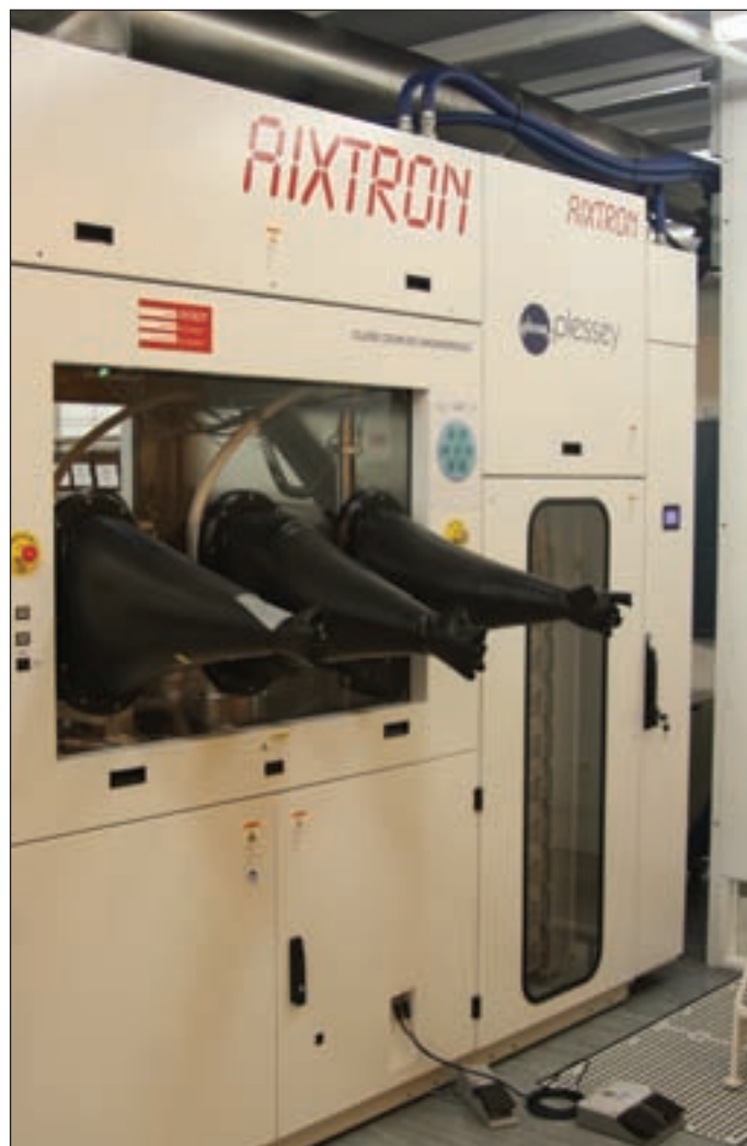
Plessey is manufacturing its GaN-on-silicon LEDs on an Aixtron reactor with a capacity of seven 6-inch wafers. The tool is fitted with various in-situ monitoring tools, which measure the curvature of the wafer and its temperature
