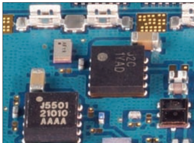
Rival semiconductors: The Javelin J5501 CMOS B1 PA alongside a BII GaAs PA (J2C) Credit: Business Wire)
