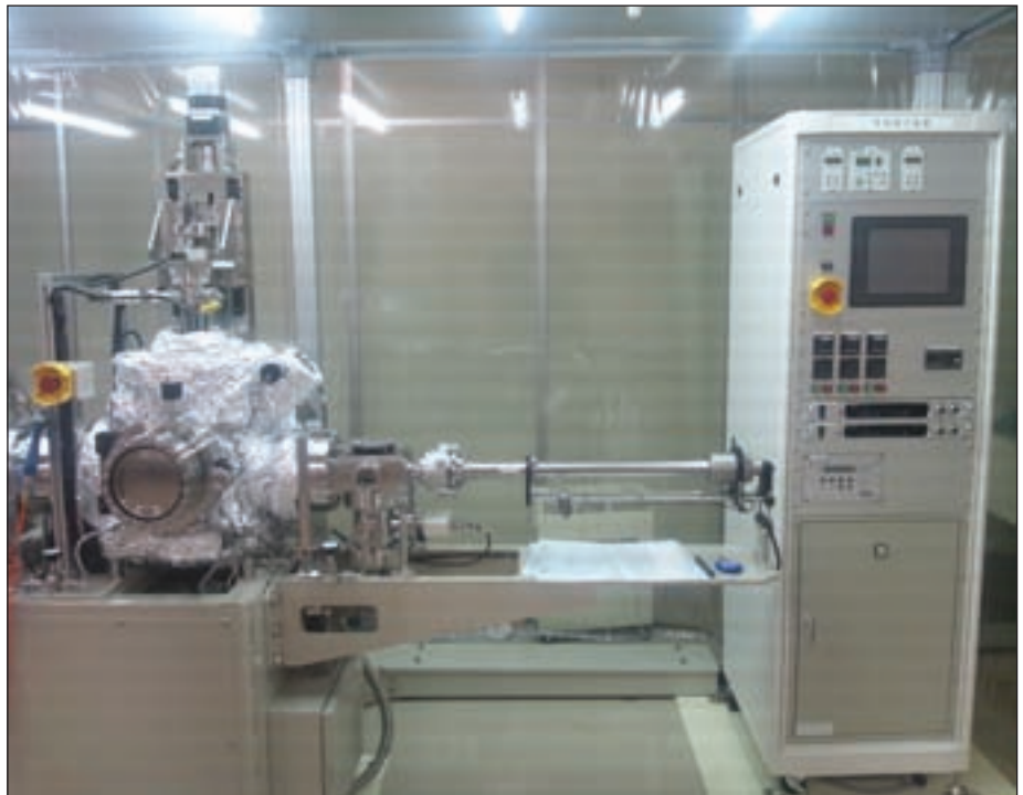
The surface-activated bonding tool involves the bombardment of substrates by a beam of fast argon atoms
