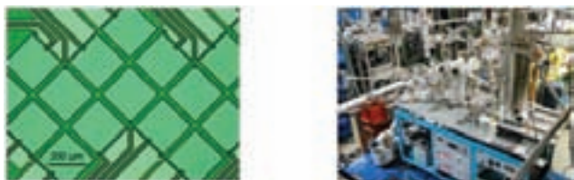
The superconducting X-ray detector developed by AIST, used to identify N dopants at a very low concentration in SiC (left) and SC-XAFS installed at a beam line of Photon Factory, KEK (right)
