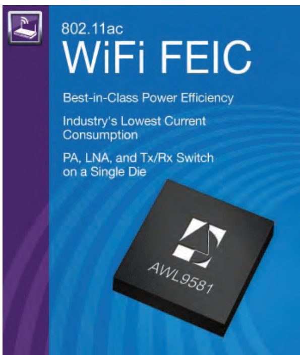
The 2.5 mm x 2.5 mm x 0.4 mm QFN packaged device
