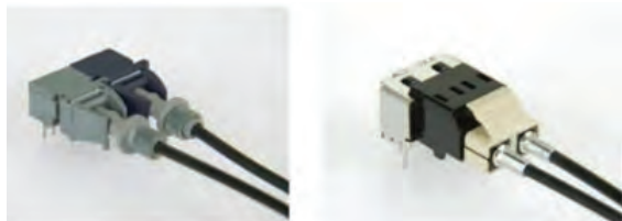
Firecomms RedLink transceiver and LC connector
