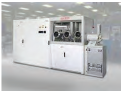
Aixtron Close Coupled Showerhead reactor
