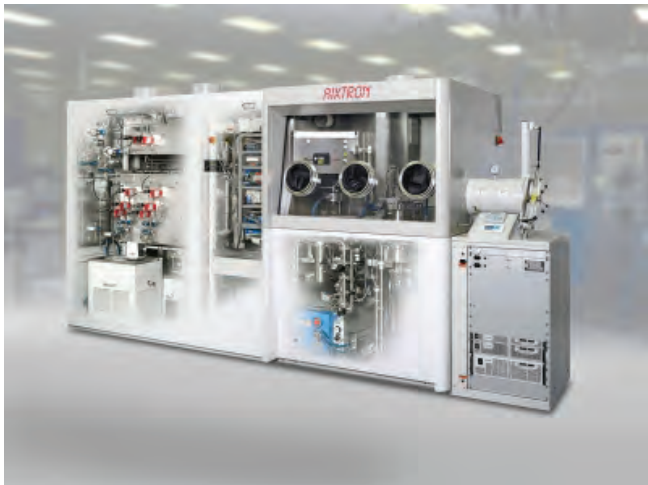
Aixtron Close Coupled Showerhead (CCS) Reactor
