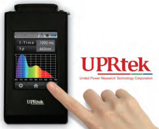
UPRtek MK-350 LED meter in “Spectrum” mode
