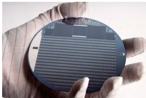
III-V multi-junction concentrator solar cells on 4-inch diameter wafer. (Credit : Fraunhofer ISE)
