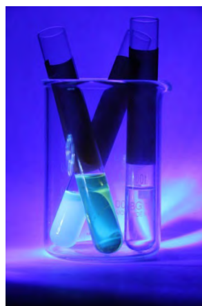
Novel cadmium selenide (CdSe) quantum dots with ligand enhancement chemistry. The vials on the left contain quantum dots; the vial on the right contains solvent without quantum dots. (Credit: Delaina Amos.)
