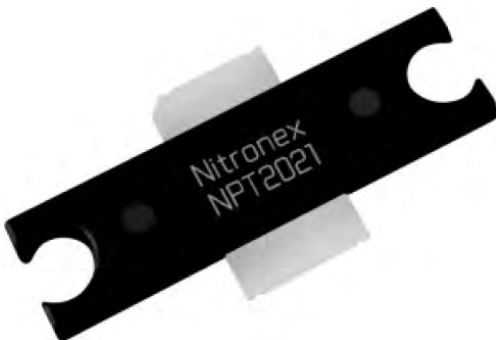
NPT2021 device in industry-standard TO272 plastic package
