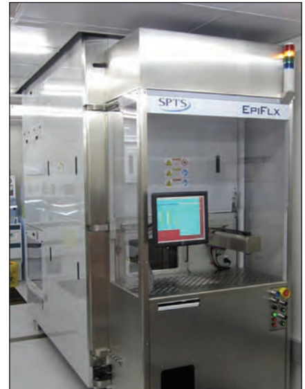
The EpiFlx reactor will extend the epitaxial growth process, pioneered at QMF, to commercial scale production of SiC coated silicon wafers
