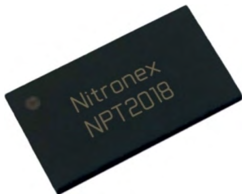
NPT2018 device in 3 x 6 DFN plastic package
