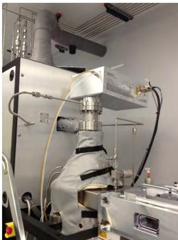
ALD system converted with a hollow cathode plasma source
