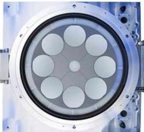
*Aixtron AIX G5 HT planetary reactor*
