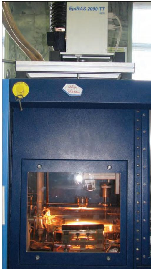
At Ioffe Physical Technical Institute, researchers produce multi-junction solar cells using an Aixtron MOCVD tool equipped with a LayTec's EpiRAS TT system. These cells have been deployed in a concentrating photovoltaic system
