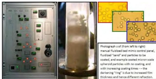
In FBCVD simple or complex shapes are coated by passing precursors over their hot (or cooled) surfaces as they are suspended in a fluidized bed of either sand or an equivalent powdered material. Heating is used when decomposing precursors and cooling is used when condensing materials such as polymers on the particles.
