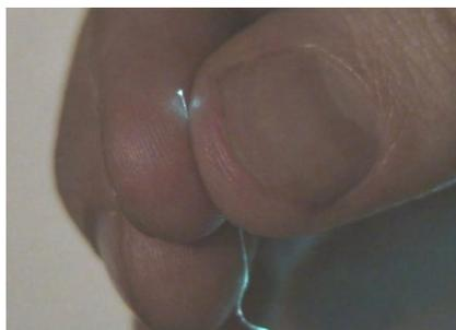
*A MicroLED coupled to an ultra-thin Plastic Optical Fibre (POF).*
