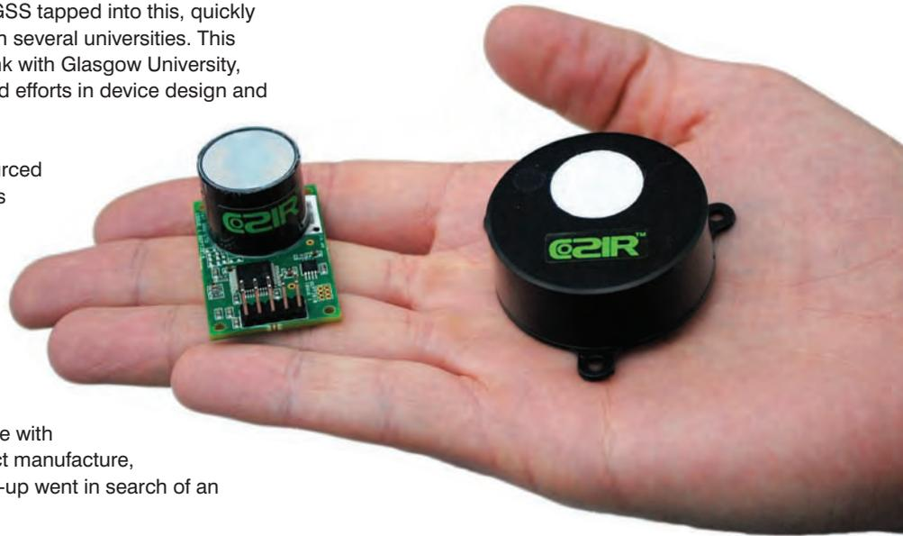
The COZIR sensors produced by GSS are a low-power product. The 20 mm path length version can detect CO<sub>2</sub> levels of 0.2 percent to 100 percent, while the 70 mm version monitors CO<sub>2</sub> levels up to 1 percent
