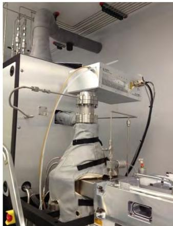
ALD system converted with a hollow cathode plasma source
