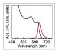
The CdTe nanodisks show a continuously tuneable PL peak position, scaling with the thickness of the disks
