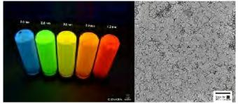
QMC's CdSe Tetrapod Quantum Dots. Left: Luminescent Vials show colour varies with QD size. Right: Tetrapod Quantum Dots by Electron Microscope
