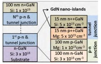
Figure 1: Epitaxial design of the cascaded p-n junctions
