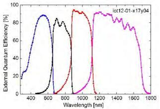
External quantum efficiency of the four-junction solar cell. The measurements were carried out at the Fraunhofer ISE CalLab In this multi-junction solar cell, several cells made out of different III-V semiconductor materials are stacked on top of each other. The single subcells absorb different wavelength ranges of the solar spectrum.
