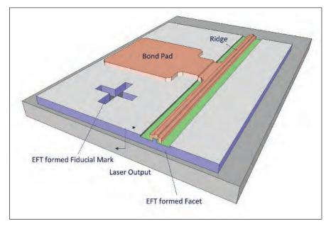
EFT can be used to etch fiducial marks to the laser and silicon photonics chip, aiding low-cost passive alignment
