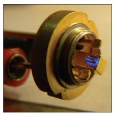
Superluminescent diodes produce a spectral output that narrows with increasing drive current
