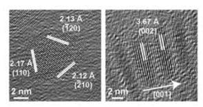
TEM micrographs showing Cu2Te (left) and CdTe (right)
