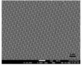
A nanowire array in the solar cell. (Photo: Eindhoven University of Technology)
