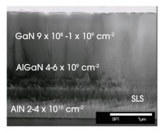
Figure 1. An scanning tunnelling electron microscopy image of an AIN/SLS/AIGaN/GaN heterostructure reveals that the dislocation density in nitride films grown by MBE can rival those found in MOCVD-grown samples
