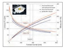
Figure 4: Electro-optical characteristics of a 1mm<sup>2</sup> ThinGaN chip in a Dragon package: device from production (blue), device with improved transport (black) and optimized epitaxial structure (orange)
