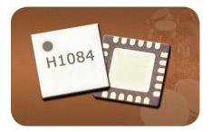
The HMC1084LC4 SP4T switch exhibits fast switching speed of 15 ns (rise and fall times) and consumes much less DC current than PIN diode based solutions. With
