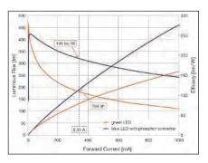
Figure 8: Current-dependent luminous flux and efficacy of two different approaches to generate green light. Whereas the green InGaN/GaN LED shows significant droop at high operating currents, a blue LED in combination with a phosphor converter yields higher efficacy and luminous flux at a typical driving current
