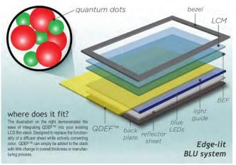
Schematic showing how QDEF works
