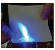
Superluminescent diodes emit a spectra with a peak at about 407 nm and an output power of 200 mW
