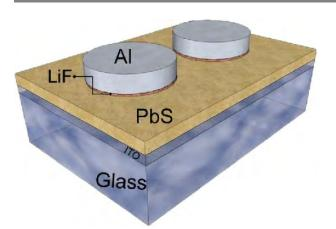
Schematic of metal-lead sulphide quantum dot Schottky junction solar cells (glass/ITO/PbS QDs/LiF/AI). Novel Schottky junction solar cells developed at NRL are capable of achieving the highest open-circuit voltages ever reported for colloidal QD based solar cell. (Photo: U.S. Naval Research Laboratory)
