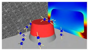
Nanoantennas made of semiconductor InAs can help scientists detect molecules with infrared light (Credit: Daniel Wasserman)
