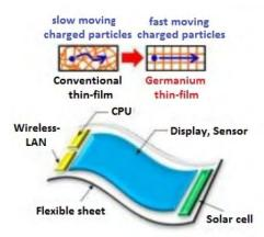
High-speed germanium thin-film transistors enable nextgeneration electronics
