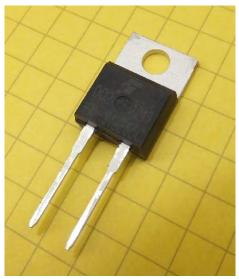
Toshiba SiC Schottky Barrier Diode
