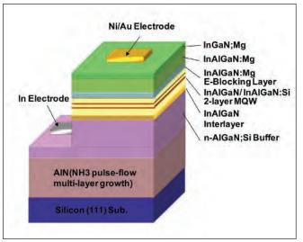
Figure 9. Moving from a sapphire substrate to one made with silicon aids the development of vertical LEDs. A damaging laser lift-off process has to be used to separate the epitaxial stack from sapphire, but with silicon a wet chemical etching approach can be employed to yield a pristine chip
