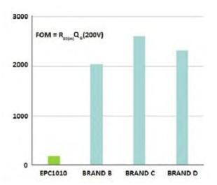
*Source: EPC Corporation* EPC Corporation is one of the leading proponents of GaN for power management applications, and they make a compelling case for this technology. In Figure 4, they illustrate the theoretical performance comparison for GaN technology versus the incumbent silicon MOSFET technology and SiC technology. *Figure 4: Theoretical "RQ" Performance*
