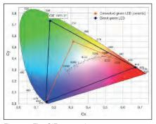
Figure 7: The CIE 1931 colour space chromaticity diagram shows two red-greenblue approaches with given red (610 nm) and blue (450 nm) LEDs used in combination with a direct green InGaN LED or a phosphorconverted green LED. The narrower emission spectra of a direct green InGaN LED, compared to green generated by phosphor conversion, makes this device better suited to projection
