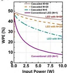
Figure 2: The change in wall plug efficiency of the modeled commercial LED (N=1) and cascaded LEDs with N=5, N=20, and N=50
