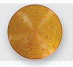
Multi-zone circuit layouts in a polyimide construction are highly customized to deliver exacting performance up to 250°C.
