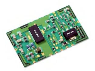
Optimised for L-Band commercial air traffic control, military radar, and long range perimeter monitoring applications at 1.2 to 1.4 GHz, MACOM's new 2-stage, fully matched GaN in Plastic power module scales to peak pulse power levels of 100W in a 14 x 24 mm package size - delivering twice the power of comparably sized competing products
