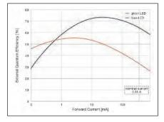
Figure 2: Comparison of the current dependent external quantum efficiency (EQE) of a blue and green 1mm<sup>2</sup> InGaN/GaN LED emitting at 442 nm and 530 nm, respectively
