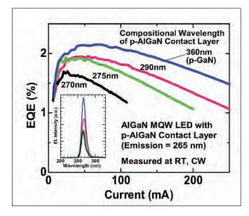
Figure 6. The aluminium composition in AlGaN can be reduced without a large impact on EQE. This indicates that an AlGaN layer, which is less absorbing than GaN, could lead to higher efficiencies in a modified device. The downside of *p*-AlGaN is a lower hole density, but this can be compensated with a better electron blocking layer. When researchers at RIKEN followed this path, their devices delivered far higher EQEs than before
