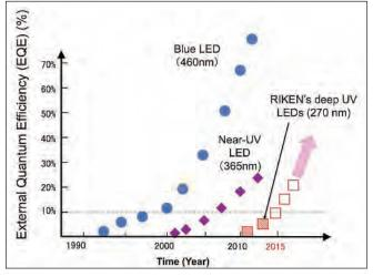
Figure 2. The efficiency of LEDs emitting in the deep UV is significantly less than that for the blue
