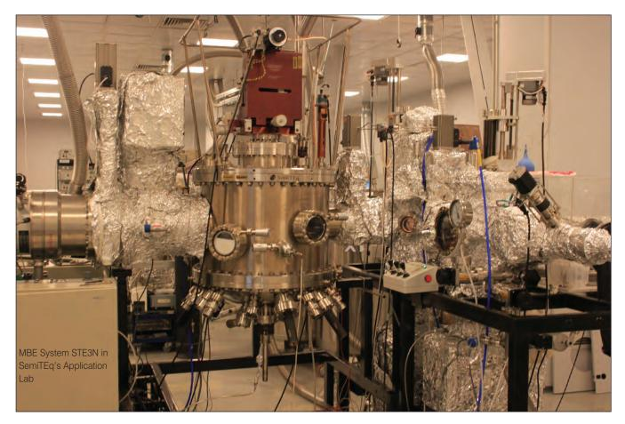
systems: the opportunity for *in-situ* monitoring offered by reflection highenergy electron-diffraction, which can be used to identify the transition from threedimensional to two-dimensional growth and provide surface reconstruction; the growth of sharper hetero-junctions; and a safer, easier route for the research and development of material systems and devices.
