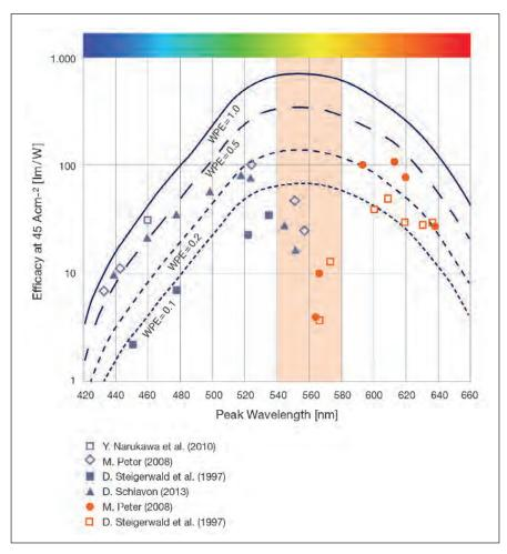
Figure 1: Efficacy of III–nitride (green data points) and III–phosphide (red data points) LEDs with different wavelengths (data taken from recent publications). The blue lines represent the CIE 1924 luminosity function multiplied by the corresponding value of the wall plug efficiency (WPE). Marked in yellow is the green–yellow range, which is not adequately covered by either the III–nitrides or the III–phosphides. This is the essence of the green gap problem
