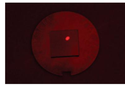
Photoluminescence is a widely used method for determining the aluminium composition in AlGaAs. Photo by James Burrus, NIST
