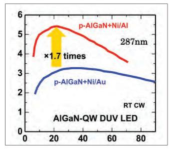
Figure 7. To take the EQE of its deep UV LEDs from about 3 percent to 5.5 percent, RIKEN's researchers used *p*-AlGaN contact layer and switched from a Ni/Au contact to Ni/Al
