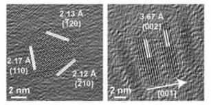
TEM micrographs showing Cu2Te (left) and CdTe (right)
