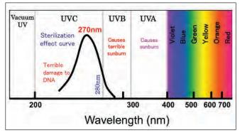
Figure 1. The ultraviolet spectrum can be sub-divided into the UVA, UVB, UVC and vacuum UV ranges. Emission at 270 nm can be used for sterilization, due to the damage that it can cause to DNA
