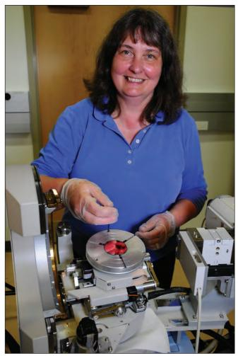
X-ray diffraction is widely used to determine the composition of aluminium in AlGaAs. Care is needed, however, because interpretation of the data must account for the substrate lattice parameter and doping-induced expansion or contraction of the lattice. Photo by James Burrus, NIST
