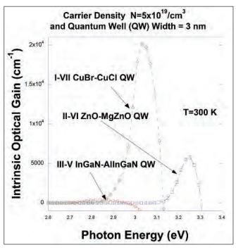
Figure 3. Optical gain spectra for CuBr/CuCl QW (green), ZnO/  $Mg_{_{0.3}}Zn_{_{0.7}}O$  QW (blue), and  $In_{_{0.2}}Ga_{_{0.8}}N/Al_{_{0.2}}In_{_{0.005}}G_{_{0.7995}}N$  QW (red) versus photon energy for carrier density of 5 x 10<sup>19</sup> cm<sup>-2</sup>
