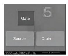
A partnership between researchers at MIT, Aixtron and the Singapore-MIT Alliance for Research and Technology have developed a gold-free process for forming ohmic contacts that involves an annealed Ti/Al/Ni/Pt stack nitrogen gas, created source and drain contacts.
