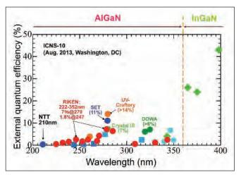
Figure 3. Some of the leading deep UV developers, including US firms Sensors Electronic Technology and Crystal IS, plus UV Craftory and RIKEN from Japan, reported EQE results at the International Workshop on Nitride Semiconductors in 2012 and ICNS 2013
