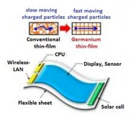
High-speed germanium thin-film transistors enable nextgeneration electronics
