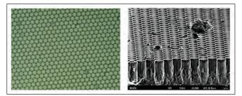
Figure 8. The array of hexagonal AIN pillars was formed by ammonia pulse-flow growth on patterned sapphire
