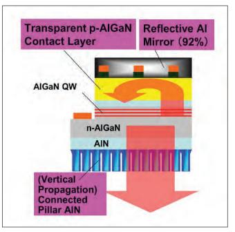
Figure 5. Light extraction in deep UV LEDs can be improved by: switching from *p*-GaN to *p*-AlGaN, a transparent contact layer; using a highly reflective mirror for this wavelength range; and forming the device on connected AIN pillars that channel light out of the chip
