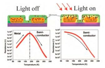
The image above shows how electrons in the gold nanorods get excited when exposed to light, then are absorbed into a thin film of zinc oxide, changing the properties of the composite from a metal into a semiconductor. (Credit: ACS Applied Materials & Interfaces)
