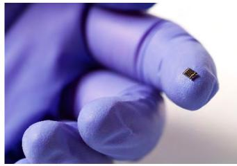
World record solar cell with 44.7 percent efficiency, made up of four solar subcells based on III-V compound semiconductors for use in concentrator photovoltaics (©Fraunhofer ISE)
