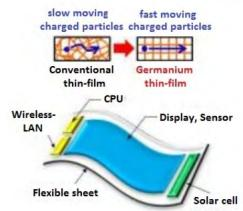
High-speed germanium thin-film transistors enable nextgeneration electronics
