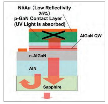
Figure 4. To enable efficient light extraction, deep-UV LEDs need to have a markedly different architecture from their blue cousins. The conventional p-type contact, GaN, absorbs UV light, which is partially reflected back into the device at AIN/sapphire and sapphire/air interfaces
