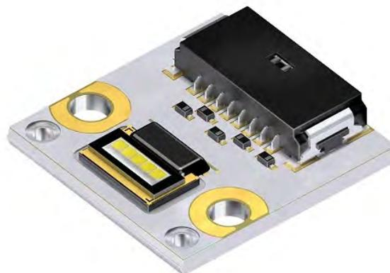
*The new variant of the Osram Ostar Headlamp Pro LED is the first multi-chip LED specifically developed for Advanced Forward Lighting Systems (Picture: Osram)*
