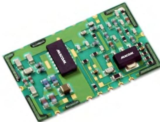
*Optimised for L-Band commercial air traffic control, military radar, and long range perimeter monitoring applications at 1.2 to 1.4 GHz, MACOM's new 2-stage, fully matched GaN in Plastic power module scales to peak pulse power levels of 100W in a 14 x 24 mm package size - delivering twice the power of comparably sized competing products*
