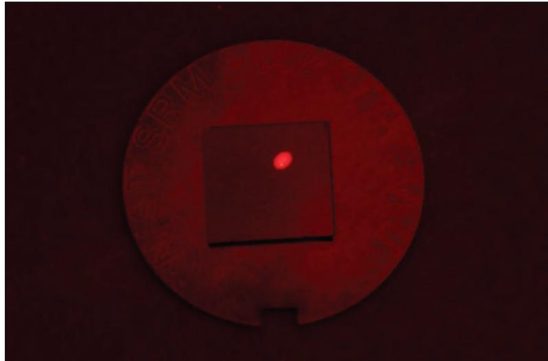
Photoluminescence is a widely used method for determining the aluminium composition in AlGaAs. Photo by James Burrus, NIST
