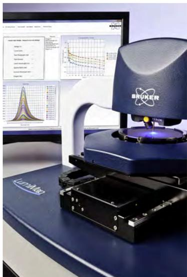
*LumiMap Electroluminescence System lights up wafer with non-destructive proprietary probe*
