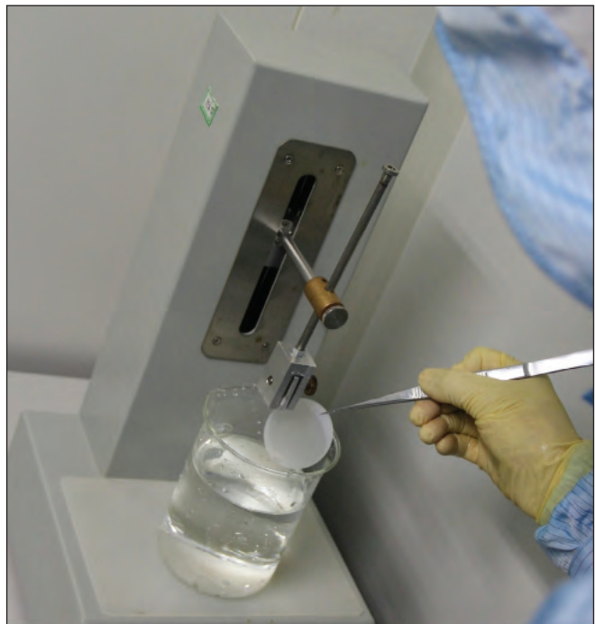
Forming nano-patterned sapphire involves dip-coating and cleaning processes
