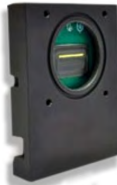
GL2048 pixel linescan camera. Tomography at 1.05 and 1.31 microns
