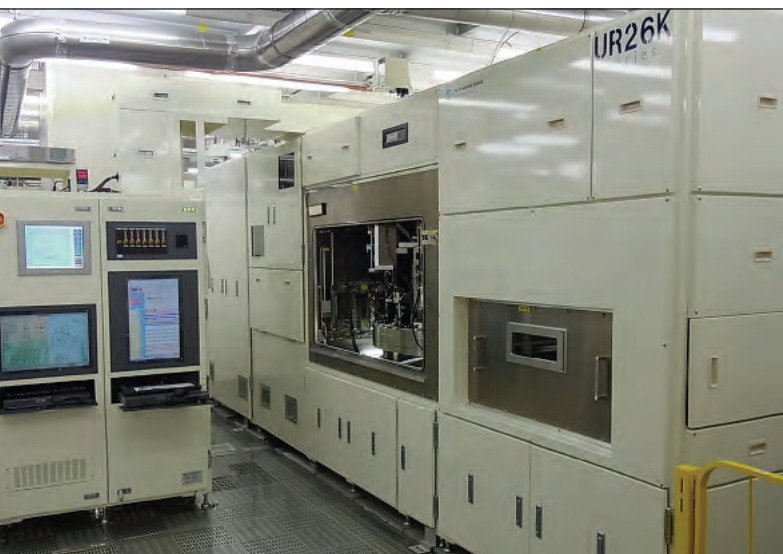
The Taiyo Nippon Sanso UR26K is the company's biggest MOCVD reactor
