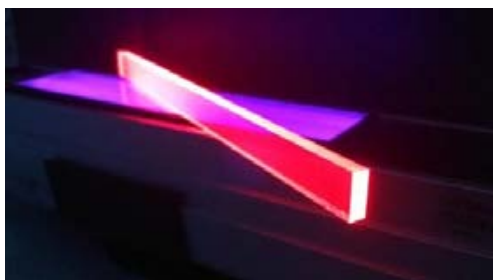
Quantum dot luminescent solar concentrator devices (embedded in the glowing pink bar) under ultraviolet illumination
