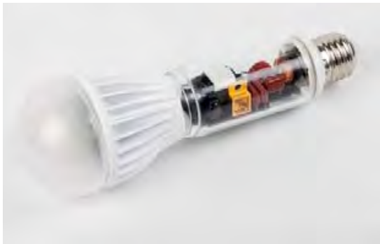
GaN transistors enable the compact design of this 2090 lumen retrofit LED lamp (exploded diagram for purpose of illustration) (Credit: Fraunhofer IAF)
