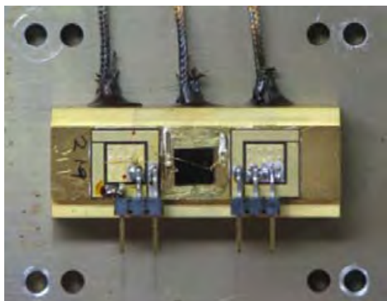
This image shows testing of a polythiophene nanofibre array grown on a copper heat sink and dried in contact with a SiC RF device simulator. (Credit: Daniel P. Resler)
