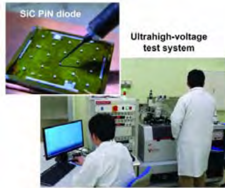
Figure 9. A fabricated diode during high-voltage testing
