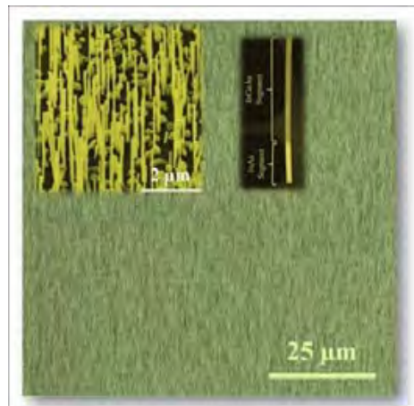
A dense array of nanowires grown directly on graphene. The insets show a higher magnification SEM view of the array and a STEM image of a single, axially heterostructured InGaAs/InAs nanowire
