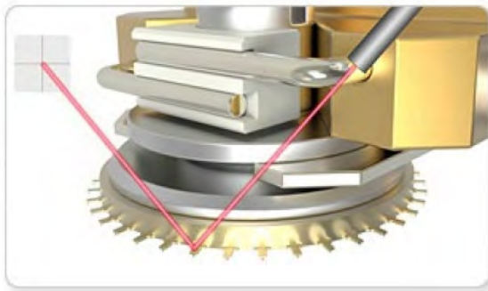
Picture: Titanium 38 Probe Revolution Cartridge NT-MDT's Titanium feature a 38-probe Revolution Cartridge for multi-probe automated cantilever replacement
