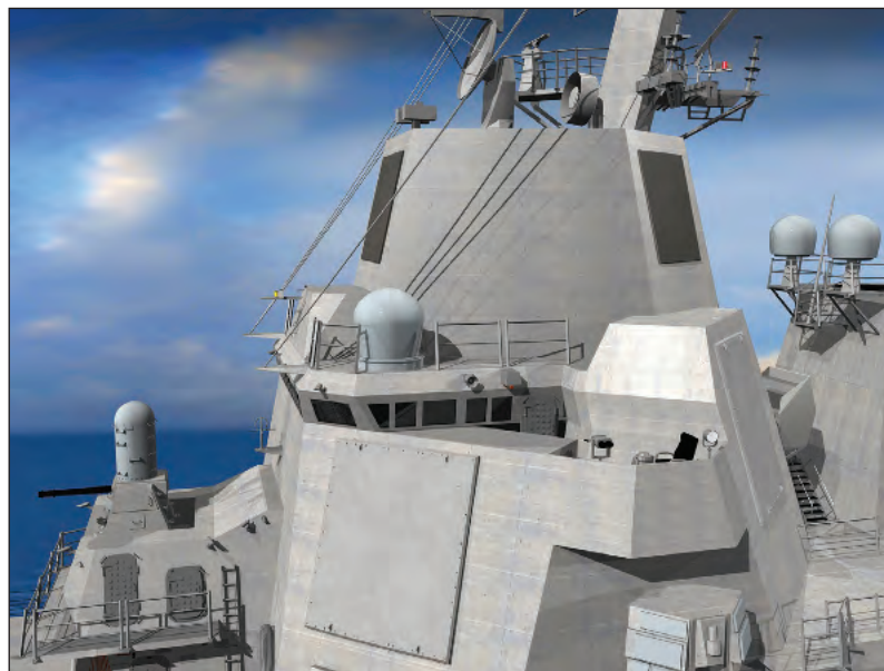
Raytheon air and defence missile radar comprises a GaN S-band radar, X-band radar and a radar suite controller. [Raytheon]
