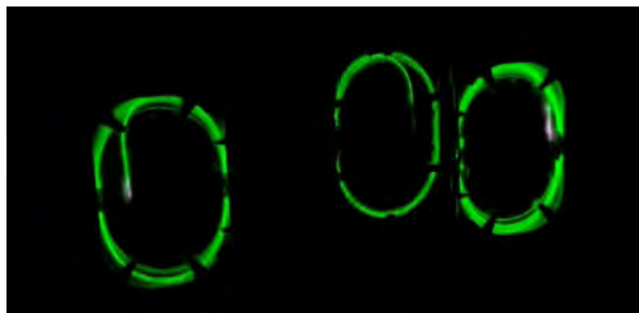
G&H space erbium doped fibre amplifier (EDFA) during radiation testing
