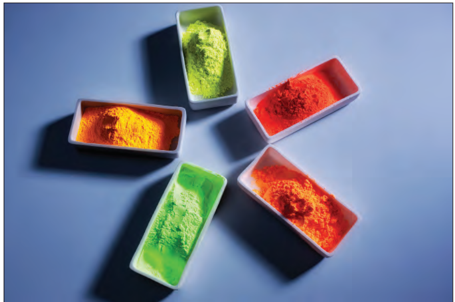
Figure 1: Intematix produces a range of phosphor materials, including those based on YAG, silicates, nitrides and aluminates.
