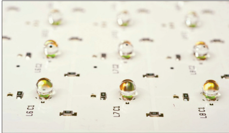
Figure 4. The fabrication of the module backplane with receivers employs processes based on surface mount technology
