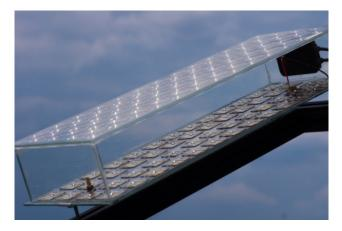
Key to this achievement was Soitec's four-junction solar cell based on wafer bonding technology and developed in cooperation with Fraunhofer ISE. This four-junction solar cell was implemented into the FLATCON module. The module aperture area, defined as the surface area of the module exposed to light, is 832 cm<sup>2</sup>. The sunlight is concentrated by a factor of 230 suns onto fifty-two 7 mm<sup>2</sup> miniature solar cells with the help of fifty-two 16 cm<sup>2</sup> Fresnel lenses.
