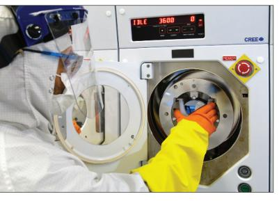
A Cree fabrication engineer removes a 100 mm SiC wafer from a spin rinse dryer, which is a fabrication tool used to clean the SiC wafer as part of the fabrication process used to make SiC MOSFETs.
