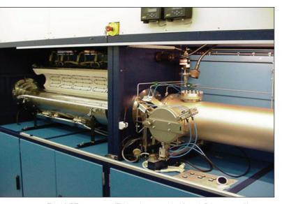
The HVPE reactor at KTH has been used to form InP layers on silicon substrates with SiO<sub>2</sub> stripes.
