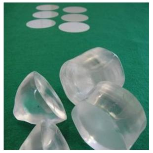
Fukuda Crystal Laboratory, based in Sendai, Japan, has created 2inch-diameter samples of ScAIMgO4 (scandium aluminum magnesium oxide) crystal, also known as SCAM. The idea is to replace sapphire in GaN-based LEDs and laser diodes by reducing crystal defects for GaNbased semiconductors grown on it. As a result, it is expected to boost brightness of GaN-based LEDs.
