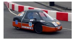
In the race, European universities to compete with innovative solutions for how far a vehicle can travel with the energy equivalent to a litre of fuel. KTH's car was fitted with thin solar cells made by Midsummer, a supplier of production lines for cost effective manufacturing of flexible thin film solar cells, CIGS (copper, indium, gallium and selenide). It came fifth.
