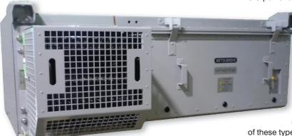
Mitsubishi's recently launched traction inverter system, which features SiC diodes and transistors, has a switching loss approximately 55 percent less than its conventional inverter system incorporating IGBTs power modules.
