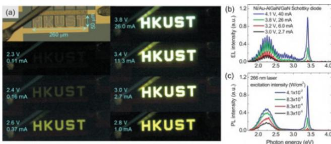
With semi-transparent Ni/Au (5/6 nm) Schottky metal, the team reported clearly seeing EL emission from the Ni/Au-Al 0.25Ga 0.75 N/GaN Schottky diode at room temperature when the forward bias is higher than 2.2V. The EL intensity becomes stronger at a higher bias.
