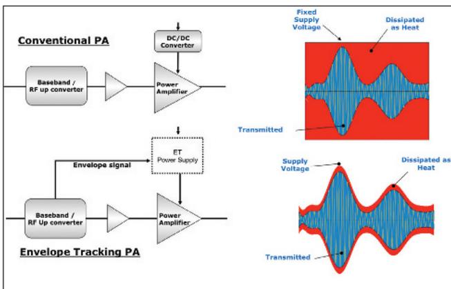
Figure 2. Envelope tracking leads to far more efficient operation of a PA, because the supply voltage is varied to give exactly what is needed at every moment in time.
