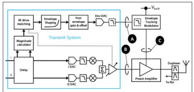
Figure 3. Envelope Tracking signal processing chain (courtesy of OpenET Alliance)
