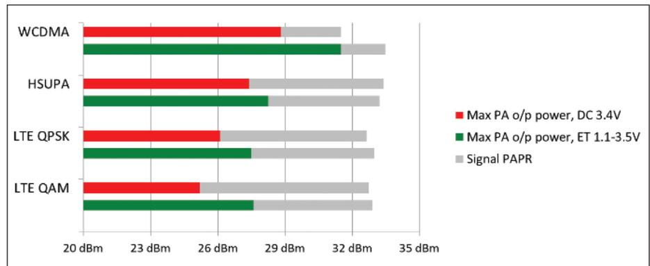
Figure 6. Maximum linear power at -38dB ACLR: optimised bias settings.
