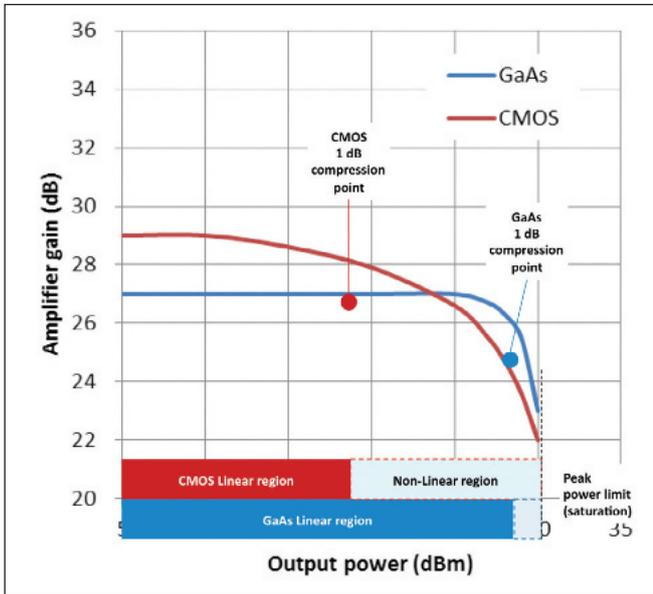
Figure 1. Power amplifiers built from GaAs deliver a linear gain over a wide range, while those based on silicon are significantly non-linear.
