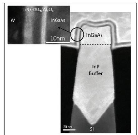
Figure 5. A dark-field, scanning tunnelling electron microscopy image of the InGaAs channel formed by imec’s engineers. The inset is a transmission electron microscopy image of the gate stack.
