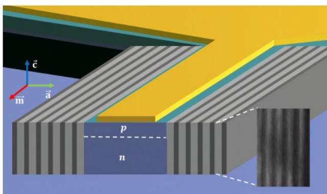
The device consists of a thin strip of gallium nitride, sandwiched between stacks of metal oxide mirrors. (In the diagram above, the mirrors
