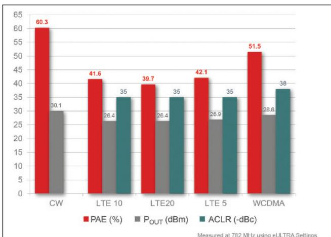
Figure 4. With W-CDMA, LTE5, LTE10 and LTE20 waveforms, Peregrine's UltraCMOS Global 1 PA shows little performance roll-off across the low band.
