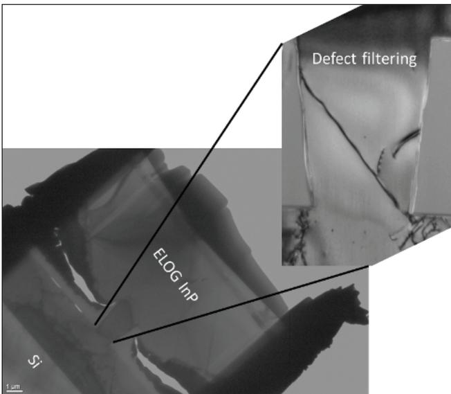
Figure 5. Cross-sectional transmission electron microscopy reveals the defect-filtering mechanism in wide openings.
