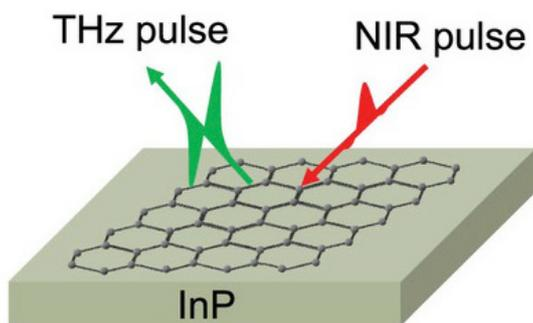
Their contactless technique involves hitting the combined material with femtosecond pulses from a near-infrared laser. The pulses excite the indium phosphide so that it emits terahertz radiation back through the graphene. Imperfections as small as a stray oxygen molecule on the graphene can then be picked up by a spectrometer.
