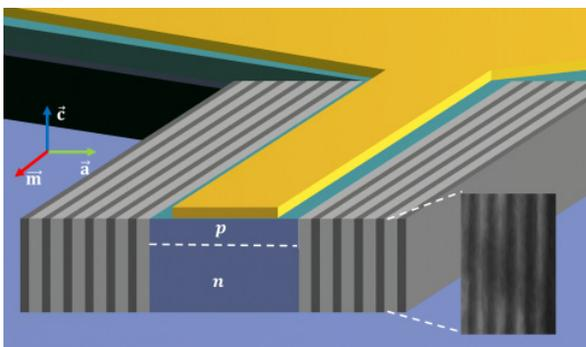
The device consists of a thin strip of gallium nitride, sandwiched between stacks of metal oxide mirrors. (In the diagram above, the mirrors are represented by the grey bars. The yellow
