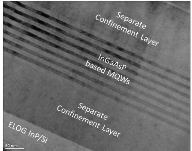
Figure 6. Transmission electron microscopy shows the high quality of the InGaAsP multi-quantum wells grown on uncoalesced ELOG InP on silicon.
