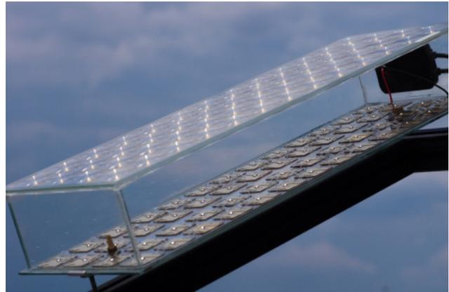
Key to this achievement was Soitec's four-junction solar cell based on wafer bonding technology and developed in cooperation with Fraunhofer ISE. This four-junction solar cell was implemented into the FLATCON module. The module aperture area, defined as the surface area of the module exposed to light, is 832 cm<sup>2</sup>. The sunlight is concentrated by a factor of 230 suns onto fifty-two 7 mm<sup>2</sup> miniature solar cells with the help of fifty-two 16 cm<sup>2</sup> Fresnel lenses.
