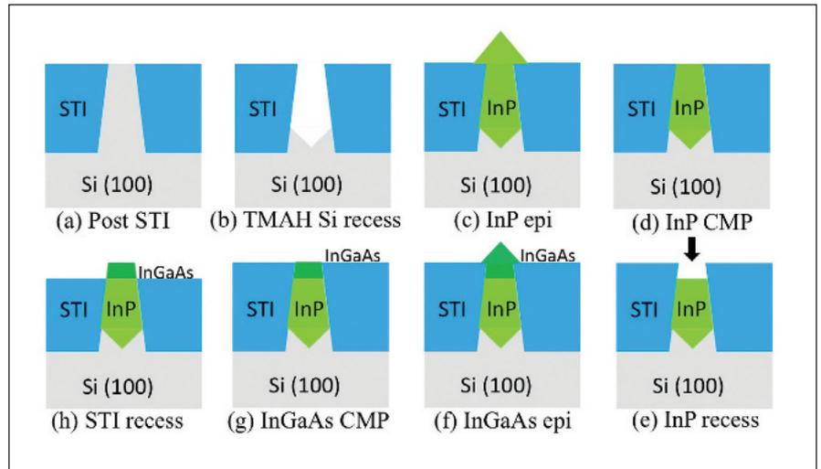
Figure 4. Researchers at imec employ aspect-ratio-trapping technology to create III-V MOSFETs on silicon with a high-quality InGaAs channel.
