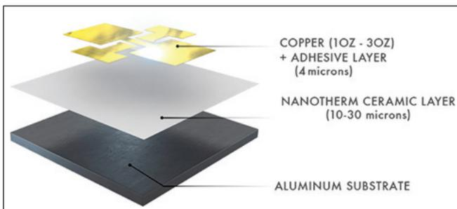
With a thin dielectric layer, Nanotherm materials have a short thermal path from the source – a semiconductor device soldered to the copper surface – to the heatsink. [Nanotherm]
