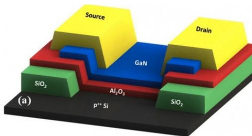
A 3D picture of the proposed TFT is shown above (a), and a scanning electron microscope (SEM) image of the top view of the device is shown below (b).
