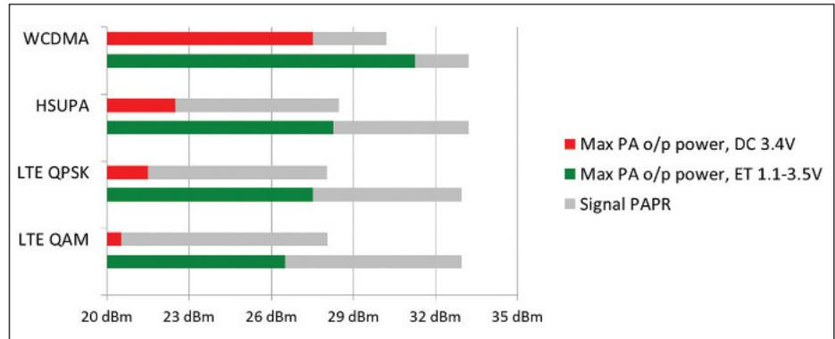
Figure 5. Values for maximum linear power at -38dB ACLR: initial bias settings. These measurements reveal that the output rises by 6 dB, or fourfold, with the introduction of ET.
