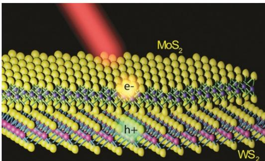
*Pictured above is an illustration of the Berkeley Laboratory's MoS<sub>2</sub>/WS<sub>2</sub> heterostructure. It shows a MoS<sub>2</sub> monolayer on top of a WS<sub>2</sub> monolayer. Electrons and holes created by light are shown to separate into different layers.*
