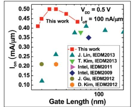
Figure 7. The MOSFET from UCSB sets a new benchmark for on-current at short gate lengths.
