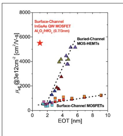
Figure 3. The surface-channel MOSFET produced by KANC produces very high mobility, while having a low equivalent oxide thickness.
