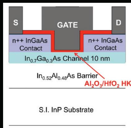
Figure 1. Researchers from KANC, working in partnership with those at Yonsei University, Sematech and GlobalFoundries, produced a MOSFET with a gate-last process that delivered an effective mobility of more than  $5500 \text{ cm}^2 \text{ V}^{-1} \text{ s}^{-1}$ .
