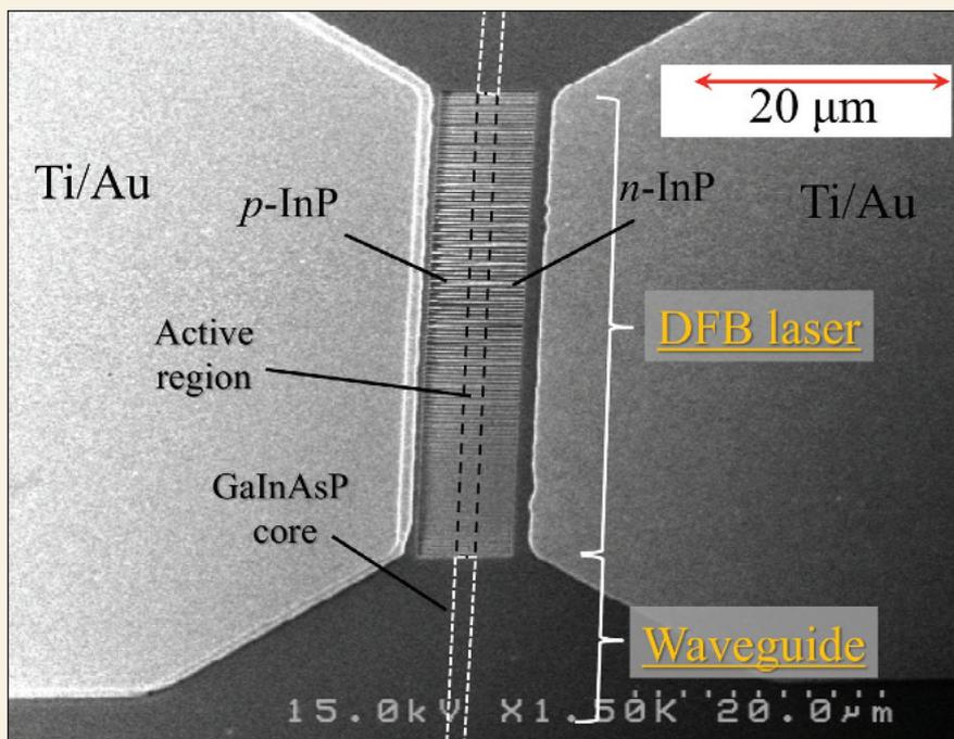
Scanning electron microscopy image of GaInAsP/InP membrane, distributed-feedback lasers integrated with waveguides and detectors.
