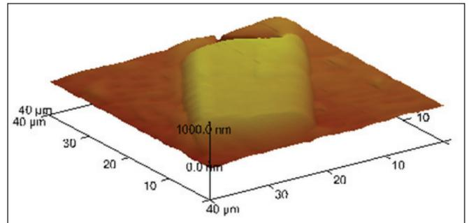
Figure 2. Atomic force microscopy reveals the high degree of flatness of coalesced ELOG InP on silicon.
