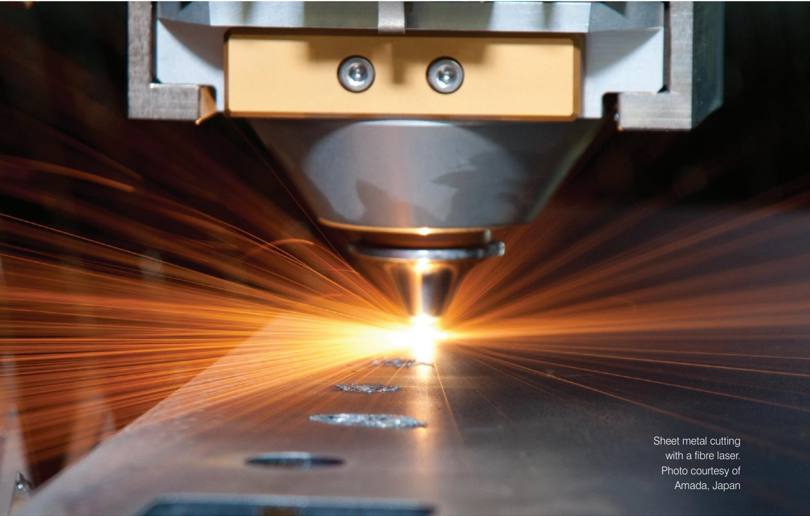
Sheet metal cutting with a fibre laser. Photo courtesy of Amada, Japan
