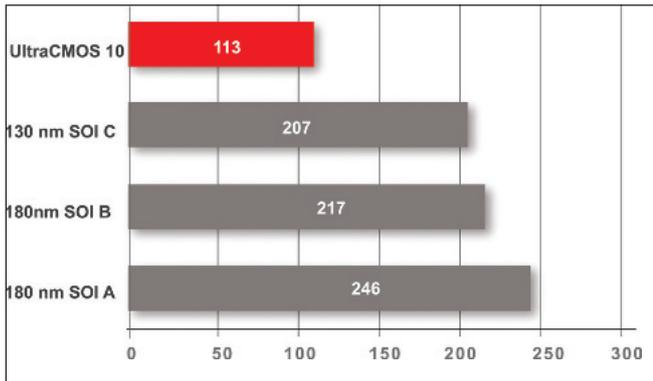
Figure 1. Peregrine's UltraCMOS 10 technology platform delivers significant performance enhancements, measured by the RonCoff figure of merit in fS.
