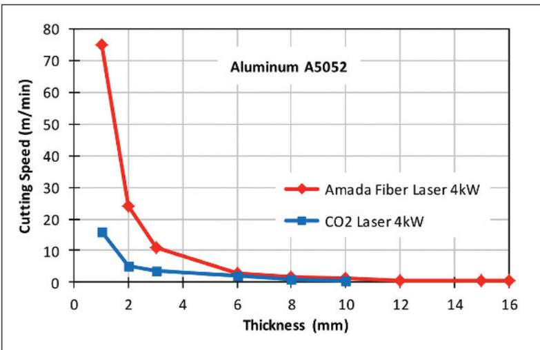
Figure 6. Cutting speed comparison for aluminium between the 4 kW Amada fibre laser and a 4kW CO<sub>2</sub> laser
