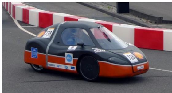
In the race, European universities compete with innovative solutions for how far a vehicle can travel with the energy equivalent to a litre of fuel. KTH's car was fitted with thin solar cells made by Midsummer, a supplier of production lines for cost effective manufacturing of flexible thin film solar cells, CIGS (copper, indium, gallium and selenide). It came fifth.
