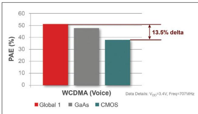
Figure 2. Peregrine's UltraCMOS Global 1 PA surpasses the leading GaAs PAs and exceeds the performance of other CMOS PAs by 13.5 percentage points. These figures are for the benchmark for PA performance of PAE (power-added efficiency) using a WCDMA (voice) waveform at an ACLR (adjacent channel leakage ratio) of -38 dBc.
