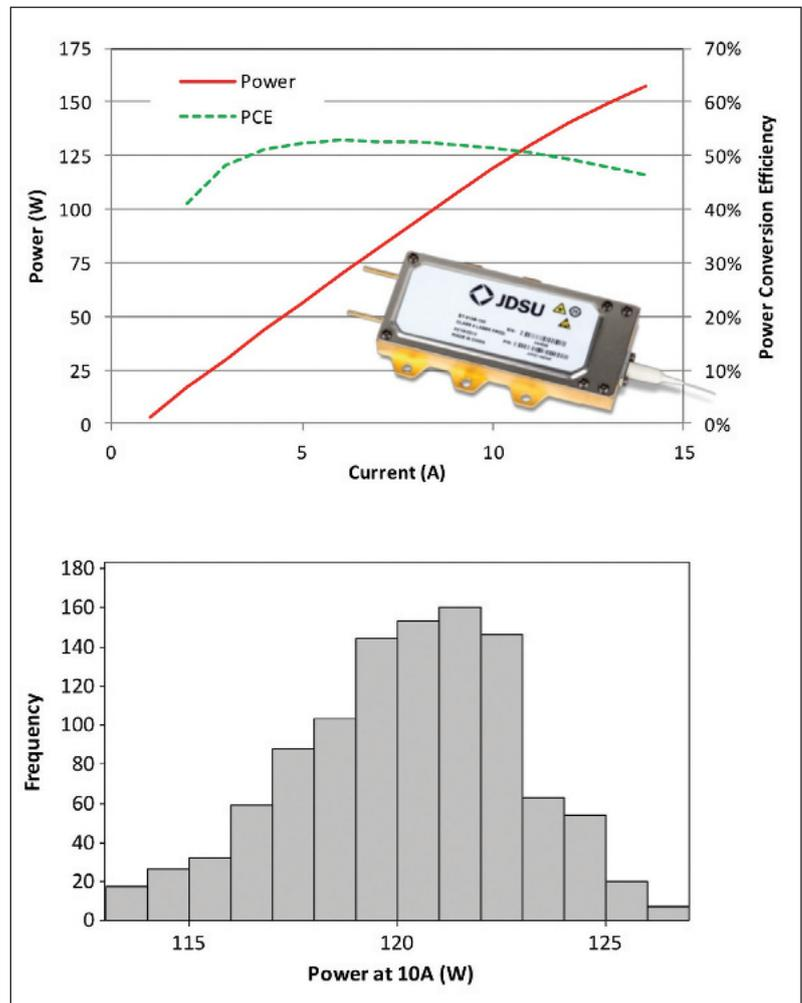
Figure 3. (a) Optical power versus drive current at 35 °C case temperature for the multi-emitter, fibre-coupled package. The laser is rated at 140 W and achieves nearly 50 percent power conversion efficiency at the rated power. (b) Optical power reading at 10 A from 1,000 units assembled. Typical optical power is about 120 W
