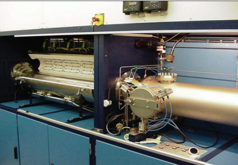
The HVPE reactor at KTH has been used to form InP layers on silicon substrates with SiO<sub>2</sub> stripes.
