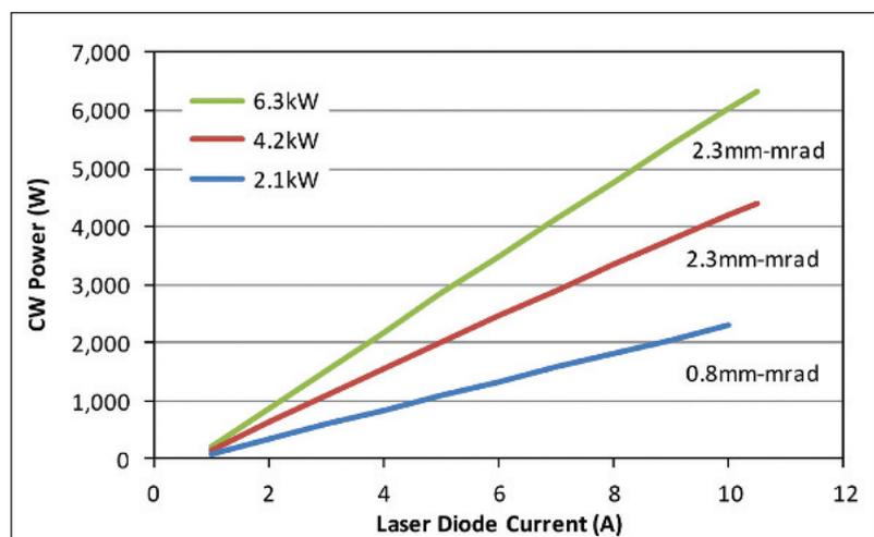
Figure 4. Fibre laser power versus pump diode current for 1-, 2-, and 3-module combined engines
