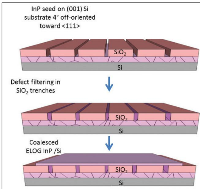
Figure 1. Epitaxial layer overgrowth holds the key to forming defect-free InP on silicon.
