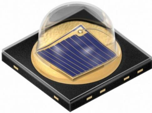
Earlier, the company also announced the 850nm Oscon Black SFH 4715A (pictured above), which boasts a typical electro-optical efficiency of 48 percent.
