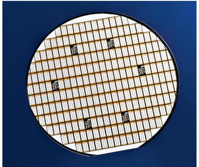
A Cree wafer containing 50 A SiC MOSFET die.
