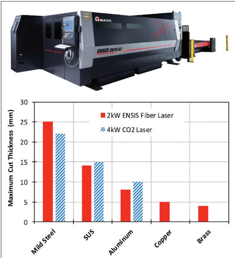
Figure 5. Maximum cut thicknesses for a variety of materials for the Amada fibre laser cutting system, ENSIS 3015 AJ, with integrated 2 kW fibre laser compared to a 4 kW CO<sub>2</sub> laser. Image courtesy of Amada
