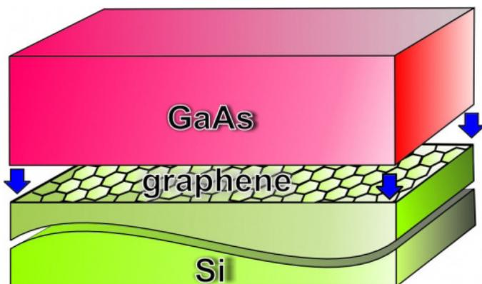
According to the researchers, the compatibility of their growth technique with current silicon planar CMOS technology presents an important step towards integrating electronics and photonics on the same chip. Applications such as photonic networks on chip, optical transceivers, free-space laser communications, and microwave photonics could benefit.
