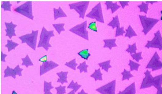
*As seen under an optical microscope, the heterostructures have a triangular shape. The two different monolayer semiconductors can be recognised through their different colours.*
