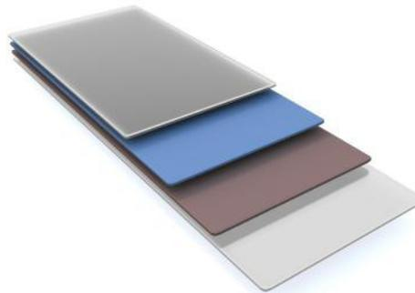
Tungsten diselenide is a semiconductor which consists of three atomic layers. One layer of tungsten is sandwiched between two layers of selenium atoms. (The image shows the two semiconductor layers in the middle, connected to electrodes on either side).
