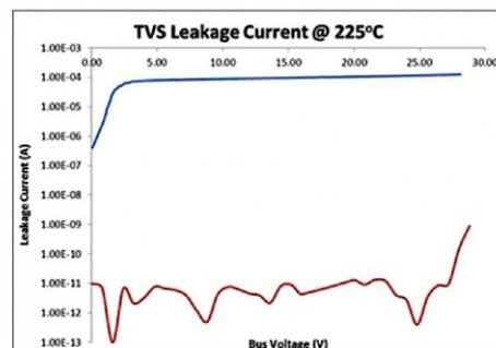
*Pictured above: Comparison of leakage currents of Si (blue) and SiC (red) TVS at 225degC. Note the several orders of magnitude lower leakage for the GE SiC device.*
