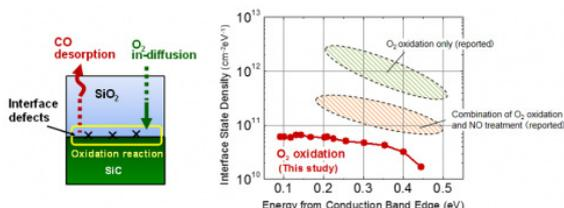
The diagrams above show: (left) a schematic of oxidation of SiC/SiO<sub>2</sub> interface; and (right) Interface state density of 4H-SiC/SiO<sub>2</sub> observed in this study, compared with previously reported typical values (hatched areas). The horizontal axis shows the energy levels of defect states referred to the conduction band edge of SiC.
