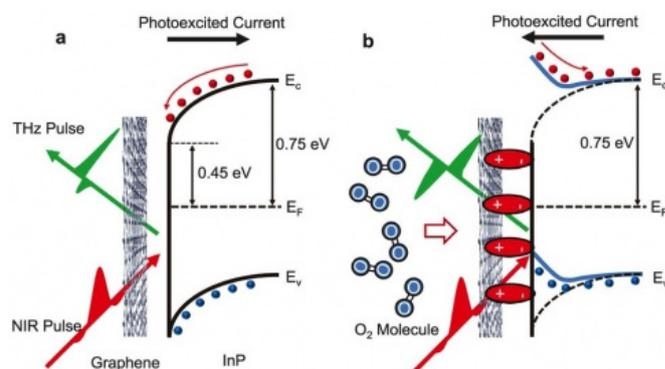
*Pictured above a), Band diagram for pristine graphene on InP. The photo excited current flows towards the substrate. (b), Band diagram for graphene on InP with adsorbed oxygen molecules between them. The charge transfer between graphene and oxygen creates dipoles, which modify the band bending. The photoexcited current now flows towards the surface.*
