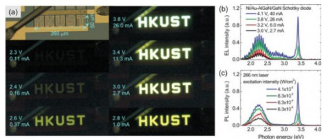
With semi-transparent Ni/Au (5/6 nm) Schottky metal, the team reported clearly seeing EL emission from the Ni/Au-Al<sub>0.25</sub>Ga<sub>0.75</sub>N/GaN Schottky diode at room temperature when the forward bias is higher than 2.2V. The EL intensity becomes stronger at a higher bias.
