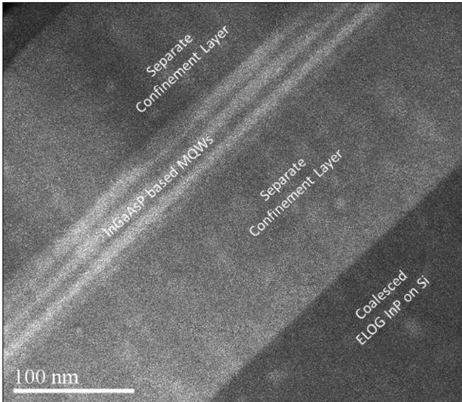
Figure 3. Cross-sectional transmission electron microscopy reveals the variations in thickness in individual layers within the InGaAsP multi-quantum wells that are formed on coalesced ELOG InP on silicon.
