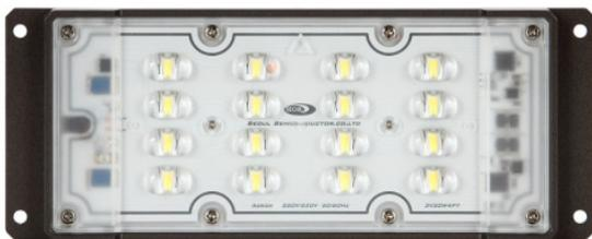
Acrich is claimed to be the first semiconductor light source that operates directly from both AC and DC power supplies. 'Acrich MJT - Multi-Junction Technology' is a proprietary family of high-voltage LEDs. The Acrich light engine does not require a complex AC/DC converter and can be operated directly from the AC mains which simplifies designs, reduces component count and improves on the reliability of the luminaire.
