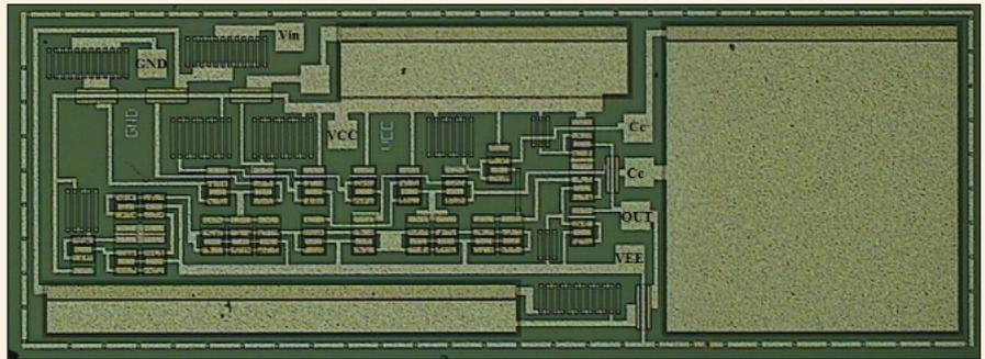
Monolithic op-amps made with 4H-SiC bipolar technology are capable of operating at 500 °C
