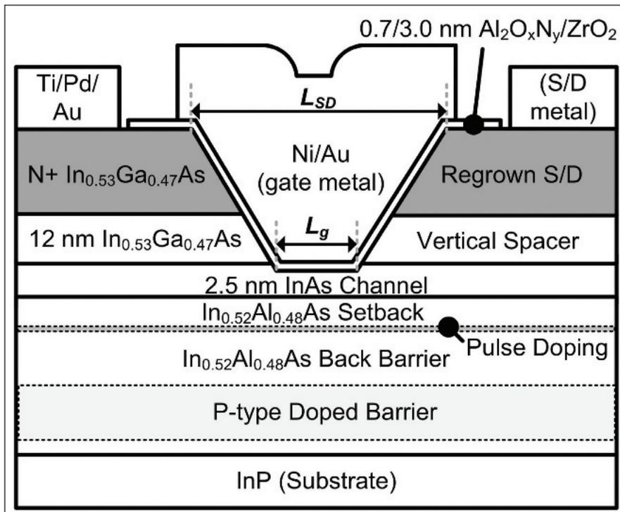
Figure 6. The vertical spacer and the thin InAs channel are claimed to hold the key to the high-performance of the UCSB MOSFET.
