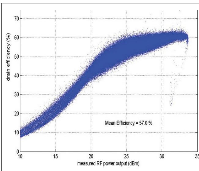
Figure 4. The measured efficiency plot of CMOS PA from dynamic supply measurements. Note that each point on this curve represents a measurement of instantaneous efficiency captured at around 100 MSPS under dynamic ET supply conditions using an LTE waveform.
