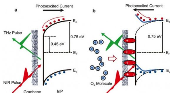
*Pictured above a), Band diagram for pristine graphene on InP. The photo excited current flows towards the substrate. (b), Band diagram for graphene on InP with adsorbed oxygen molecules between them. The charge transfer between graphene and oxygen creates dipoles, which modify*
