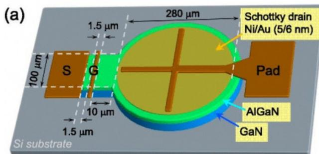
The team used an AlGaIn/GaN heterostructure consisting of a 21nm Al<sub>0.25</sub>Ga<sub>0.75</sub>N barrier and 3.8μm GaN buffer, grown by MOCVD on a 4inch p-type S (111) substrate. The heterostructure contained a 2DEG channel of density 10<sup>13</sup>/cm<sup>2</sup> and mobility 2080cm<sup>2</sup>/V<sup>-1</sup>s<sup>-1</sup> at room temperature.
