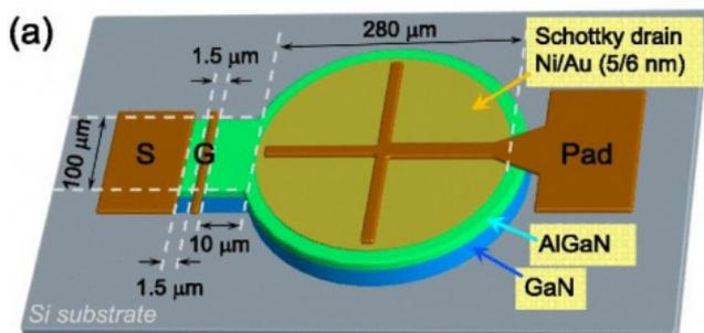
The team used an AlGaIn/GaN heterostructure consisting of a 21nm Al<sub>0.25</sub>Ga<sub>0.75</sub>N barrier and 3.8μm GaN buffer, grown by MOCVD on a 4inch p-type S (111) substrate. The heterostructure contained a 2DEG channel of density  $10^{13}/\text{cm}^2$  and mobility  $2080\text{cm}^2/\text{V}^1\text{s}^{-1}$  at room temperature.
