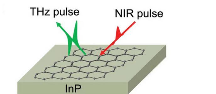
Their contactless technique involves hitting the combined material with femtosecond pulses from a near-infrared laser. The pulses excite the indium phosphide so that it emits terahertz radiation back through the graphene. Imperfections as small as a stray oxygen molecule on the graphene can then be picked up by a spectrometer.
