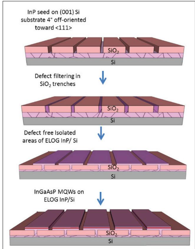
Figure 5. Turning to a new ELOG process led to the formation of un-coalesced large areas of InP on silicon.
