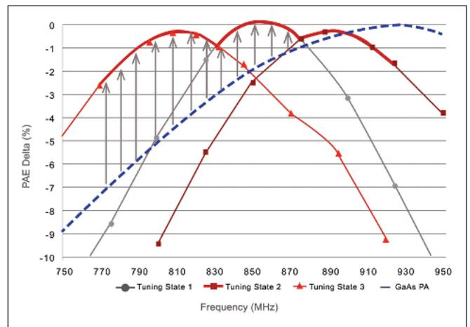
Figure 3. Peregrine's UltraCMOS Global 1 PA enables performance optimisation through tuneable matching networks; band-specific tuning provides additional rejection to other frequency bands, which helps mitigate some of the difficult interoperability cases.
