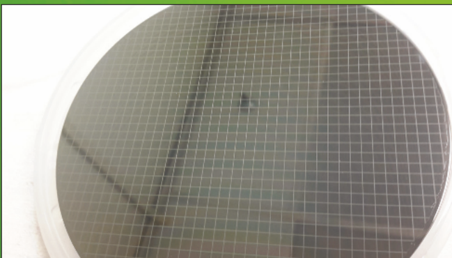
An Anvil wafer: researchers have grown cubic GaN layers on the cubic SiC-on-silicon wafers
