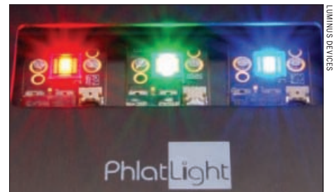
Backlight LEDs from Luminus Devices featured in Samsung and Sharp TVs at the annual CES.
