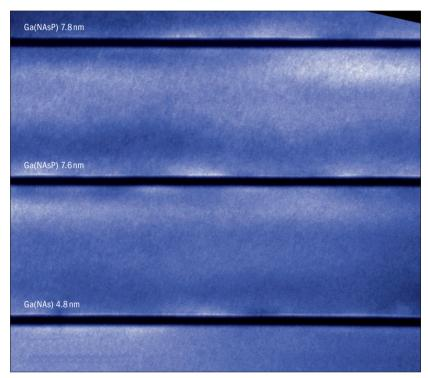
**Fig. 1.** A dark-field transmission electron microscopy image of the heterostructure containing GaNAsP wells and GaP barriers reveals no dislocations or inhomogeneous strain relaxation.
