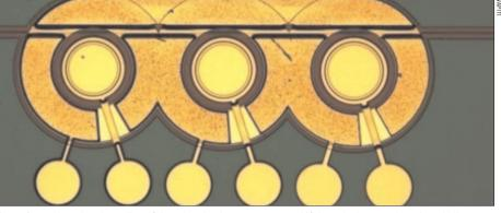
**Three rings:** changing the radius of the microring lasers creates a shift in emission wavelength and allows wavelength multiplexing for high data-rate transmission. The result should be smaller optical transceivers.
