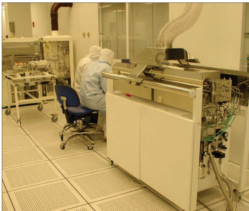
Peide Ye's team at Purdue University is producing inversion-mode InGaAs MOSFETs with minority carrier currents of more than 1 A/mm. These transistors feature gates made from Al 2 O 3 , HfO 2 and HfAlO dielectrics, which are grown by atomic-layer-deposition in an ASM ALD F-120.
