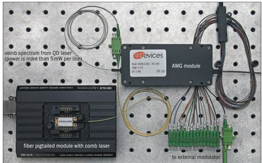
Fig. 4. Many of Innolume's initial optical experiments involved the demultiplexing of a comb laser by a commercial C-band (1550 nm), 50 GHz spacing arrayed waveguide. The O-band arrayed waveguide grating output of combs centered at 1280 and 1310 nm shows negligible power loss.
