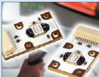
blue LEDs produce 31.4 mW at the same drive current, which equates to a wall-plug efficiency of 51%.
