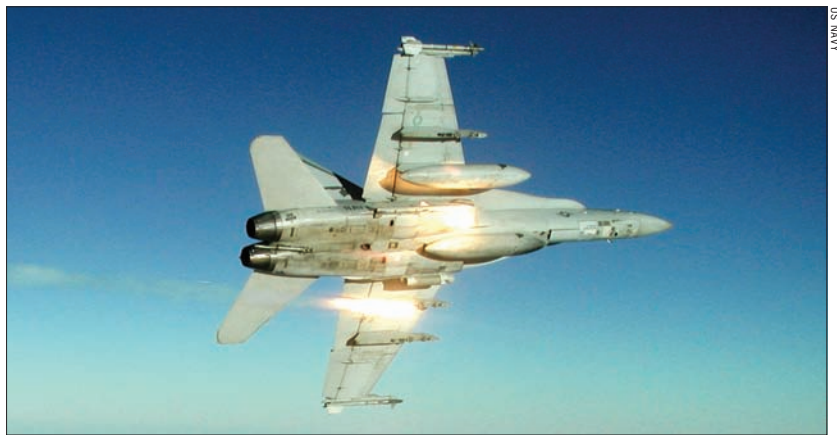
A US F/A-18 "Hornet" fires flares during a training mission. The flares form part of the fighter aircraft's defense against surface-to-air and air-to-air infrared heat-seeking missile attacks. The flares aren't always a successful decoy, however, so the Navy is funding research into mid-infrared III-V laser diodes that could be used to jam the missile-guidance systems more effectively.
