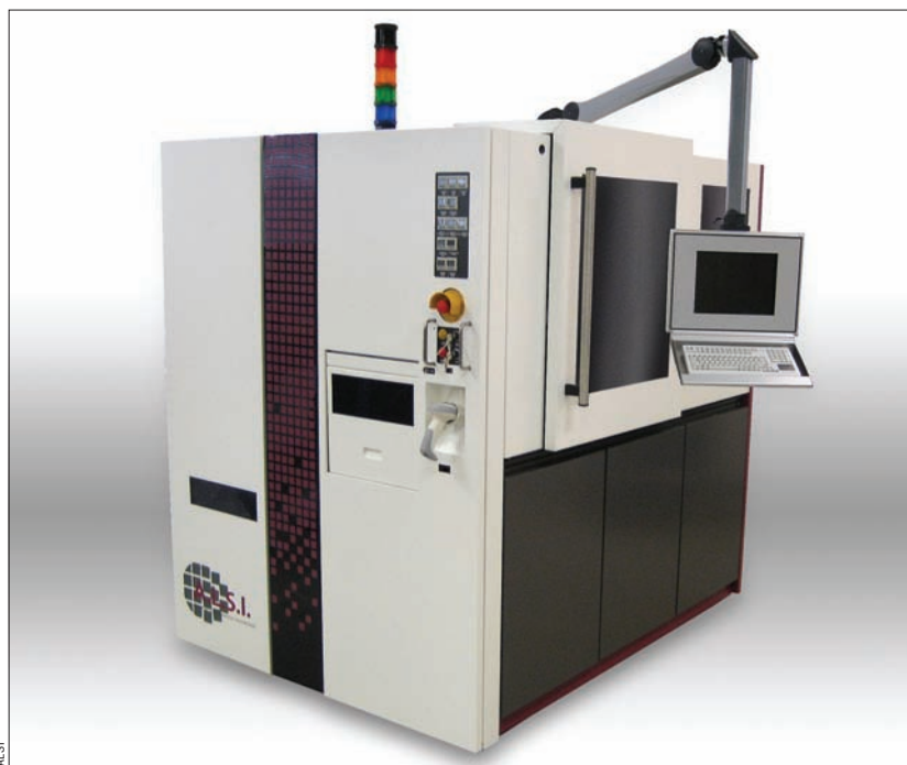
The DCA 802 automatic laser dicing system from Advanced Laser Separation International has virtually cornered the market in GaAs wafer dicing by laser. The system is based on technology developed initially at Philips and shares certain aspects of design with ASML lithography systems.
