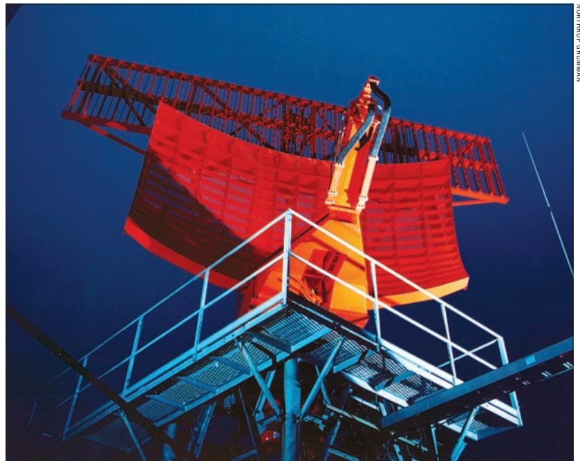
Solid-state digital airport surveillance radar , like this one from Northrop Grumman, is one example of the S-band radar applications being targeted by RFMD's 400 W GaN power amplifier.
