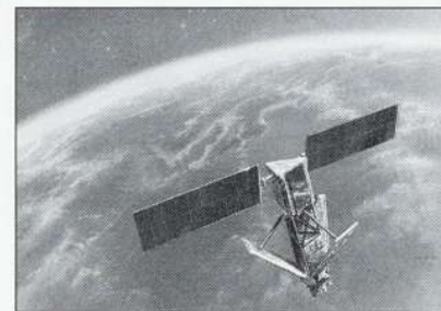
On the cover: Artist's rendition of an Iridium satellite, built by Lockheed Martin. Motorola plans to launch 66 of these satellites - all powered by GaAs-on-Ge solar cells - to construct a new wireless communications network.
