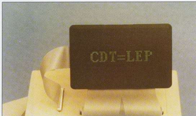
An example of a polymer LED dot matrix display produced by CDT.
