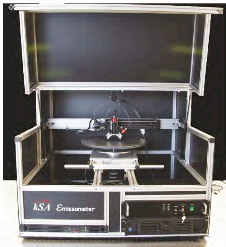
Figure 1. The kSA Emissometer, with its lid open, measuring the emissivity of a loaded Veeco K465i carrier.
