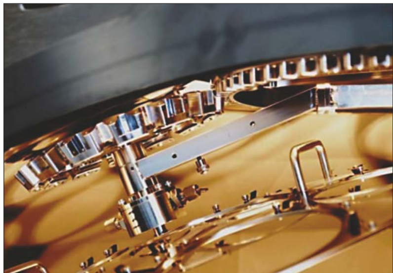
Figure 6. The HULA wafer holder assembly cuts particle generation, thanks to a magnetic drive system.
