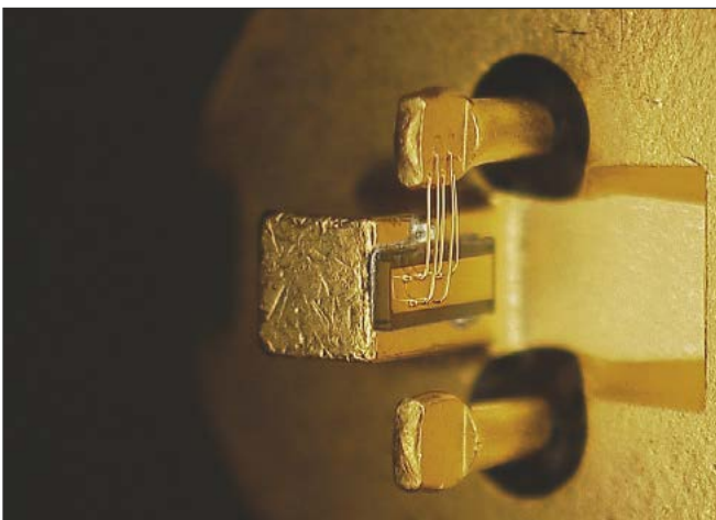
The superluminescent diode is not overwhelmed by droop, thanks to stimulated emission. Credit: S. Stańczyk, Unipress
