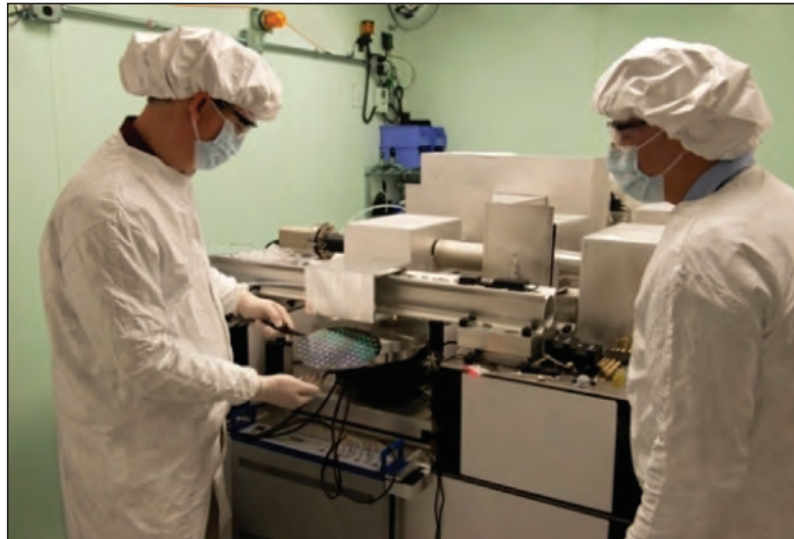
Bryan Barnes (left) and Rick Silver (right) load a wafer into the NIST-built 193 wavelength microscope
