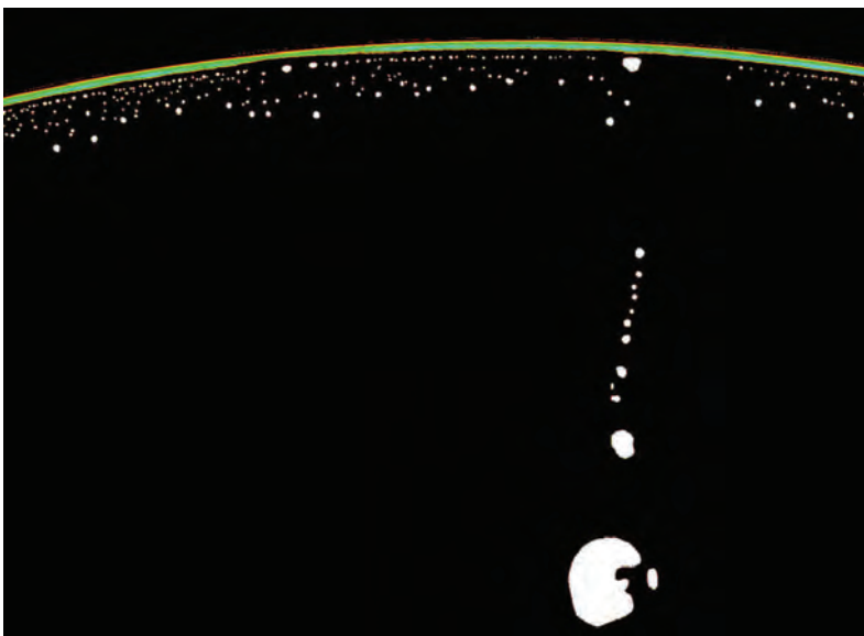
Figure 4. Acoustic image of one portion of a direct bonded wafer pair shows size variation in the voids between the wafers
