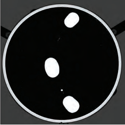
Figure 2. Acoustic image of two bonded MEMS wafers. White regions are voids between the wafers.
