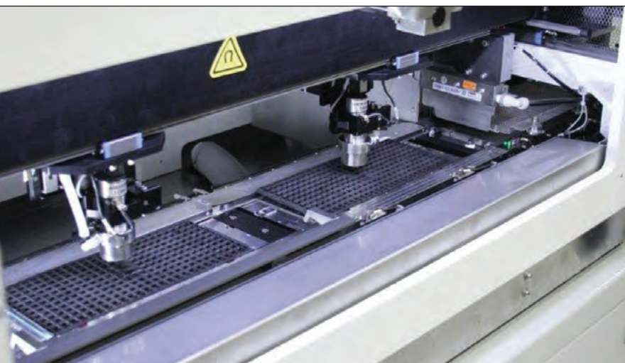
Figure 1: Automated acoustic micro imaging tools (here the Sonoscan DH2400) use carefully defined standards to make good accept/reject decisions on large numbers of components.
