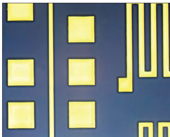
Gold plating by the Solstice S8 system
