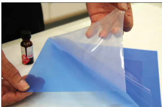
Figure 8: Photo of a CV film adhesive, a high consistency silicone calendered out to 0.012" with fiberglass scrim reinforcement embedded. Also, small bottle of Part B Activator
