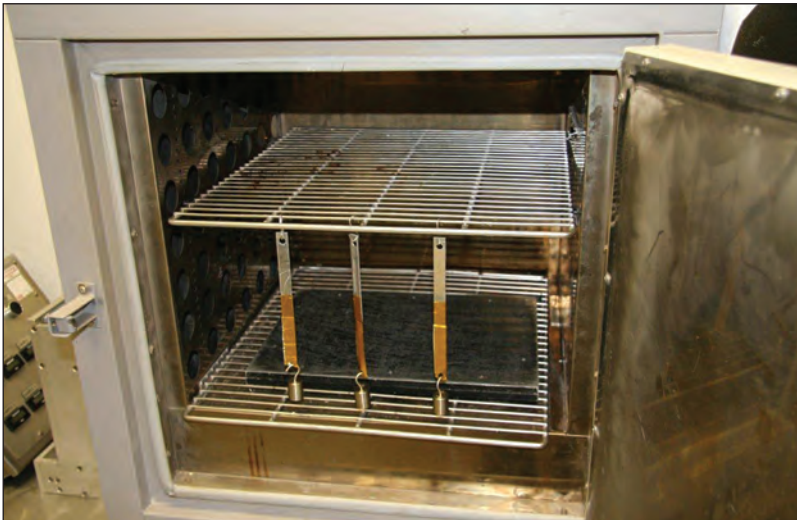
Figure 5: Static Shear Test; PSA coated onto Kapton and bonded to aluminium panels
